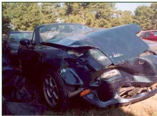
**Figure 1. Frontal damage to the 1997 Mazda Miata.**
