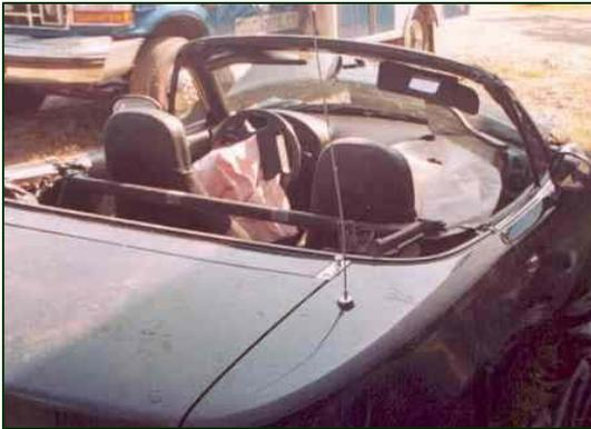
**Figure 14. Deformed front right air bag module cover flap.**
