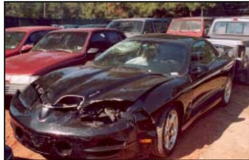
**Figure 12. Frontal damage to the Pontiac Trans Am.**
