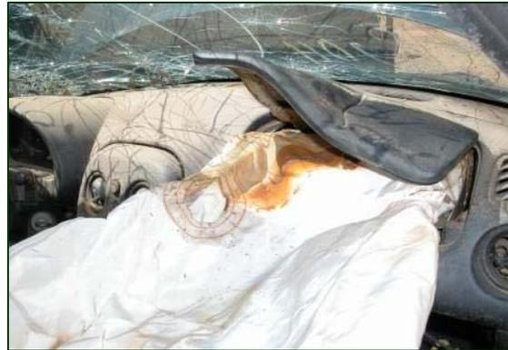
**Figure 15. View of the deformed cover flap at the time of the SCI investigation.**
