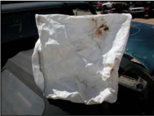
**Figure16. Deployed front right passenger air bag.**
