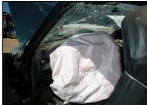
**Figure 13. Deployed driver's air bag.**
