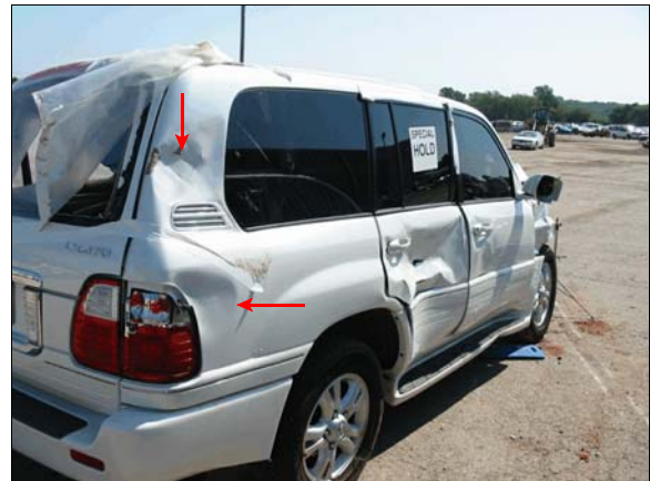
Figure 9: Overview of damage to right rear corner of LX 470 (arrows) due to impact with back of case vehicle
