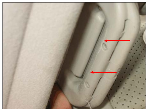
Figure 27: Abrasions on the case vehicle driver's D-ring (arrows)
