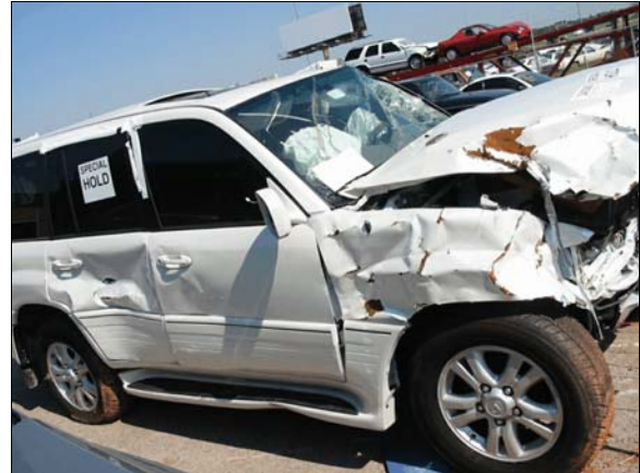
Figure 7: Damage to right side doors of LX 470 from impact with case vehicle's left quarter panel
