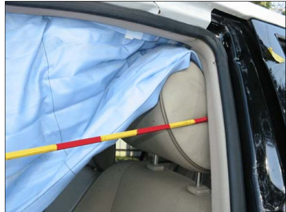
Figure 21: Case vehicle driver's head restraint obstructing driver's side curtain air bag
