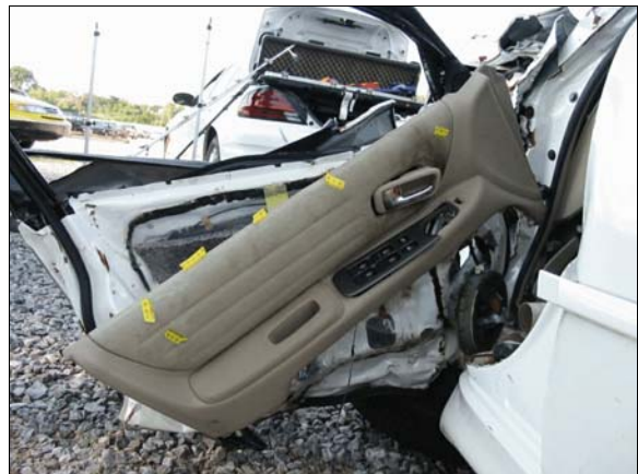
Figure 30: Occupant contact to case vehicle's left front door (door has also been damaged from rescue activities)
