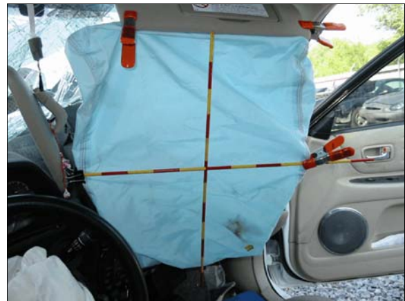
Figure 26: Case vehicle's front right air bag; each stripe on the rods is five centimeters (two inches)
