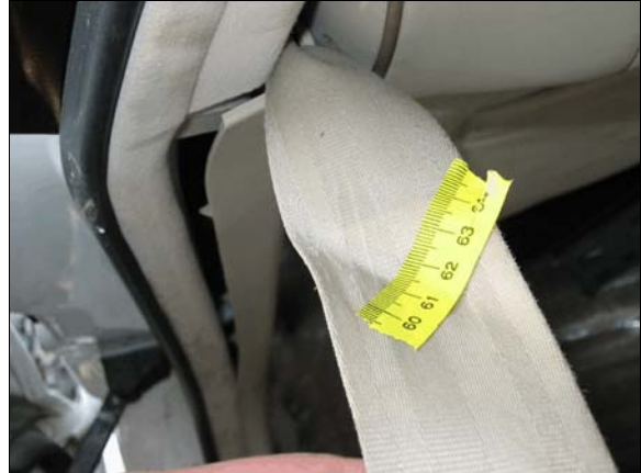
Figure 28: Case vehicle driver's shoulder belt, its stretched and abraded
