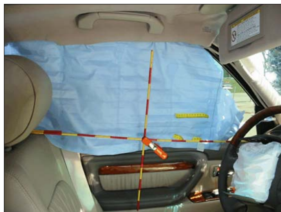
Figure 34: Driver's portion of the LX 470's left side curtain air bag, yellow tape shows possible driver occupant contact scuff on air bag
