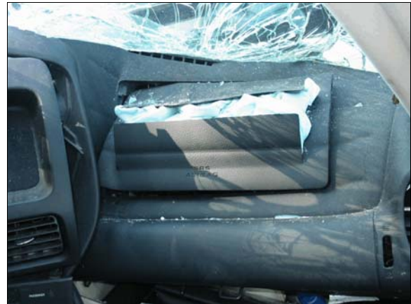
Figure 25: Case vehicle's front right air bag module flaps
