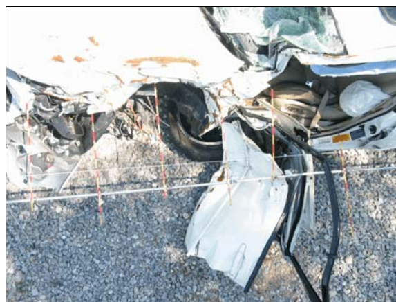
Figure 11: Top view of crush to case vehicle's left front side (driver's door also damaged by rescue activities), each increment on rods is 5 cm (2 in)
