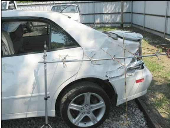
Figure 6: Damage to case vehicle's left quarter panel due to impact with LX 470's right side doors
