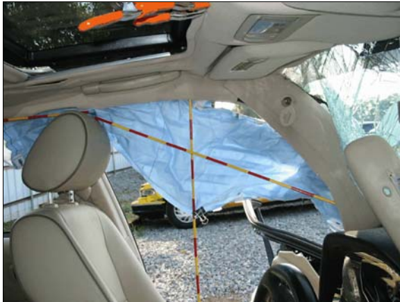
Figure 20: Overview of case vehicle driver's side curtain air bag
