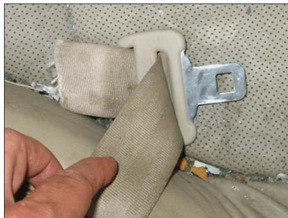
Figure 32: Case vehicle driver’s seat belt has been cut in two
