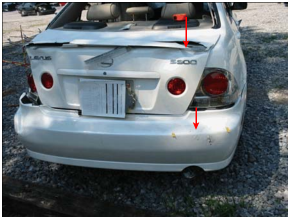
Figure 8: Damage to right portion of case vehicle's back bumper and trunk lid (arrows) from impact with the right rear corner of the LX 470
