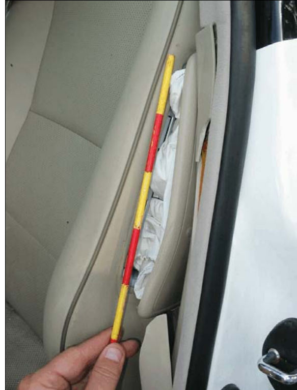
Figure 18: Case vehicle driver's seat-mounted side air bag module flap; each increment on rod is 5 cm (2 in)
