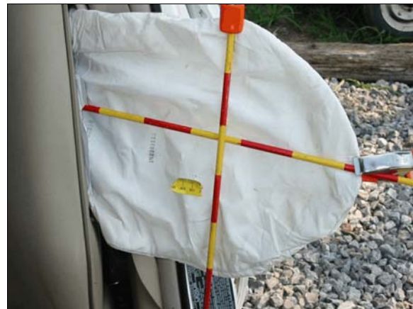
Figure 19: Case vehicle driver's seat-mounted side air bag
