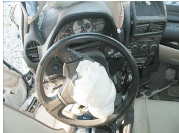
Figure 15: Case vehicle's steering wheel, lower left air bag module flap and air bag, steering wheel rotated right about 90 degrees
