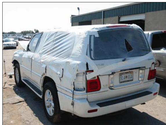
Figure 10: Overview of rollover damage to left side of Lexus LX 470
