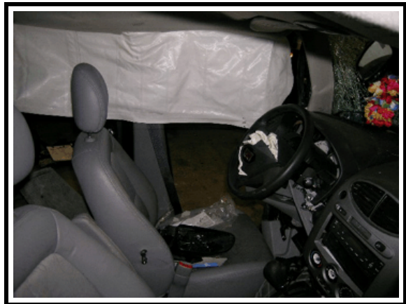
Figure 8. Driver's head curtain side air bag
