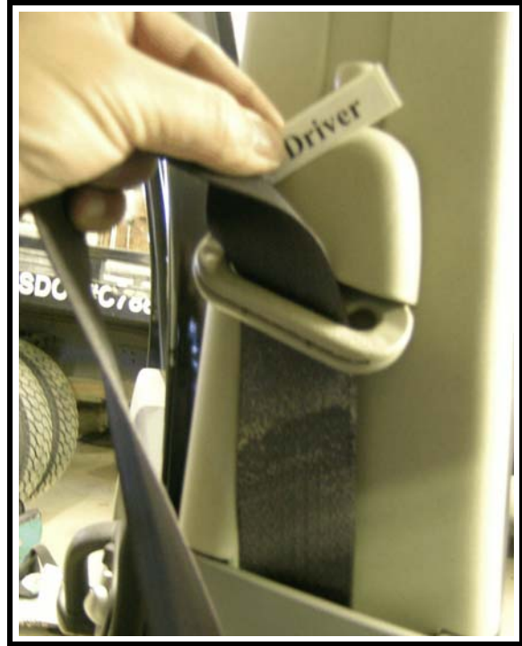
Figure 5. Loading to driver's seat belt
