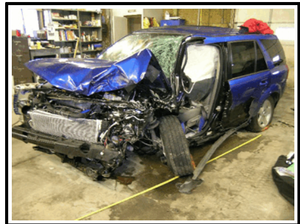
Figure 2. Front, left three-quarter view showing frontal deformation and “snagged” left front tire of case vehicle
