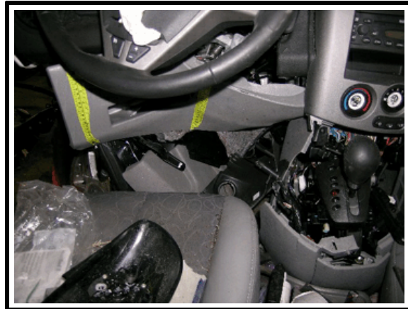
Figure 9. View showing intrusion at drivers position and lower extremity contacts to deformed knee bolster
