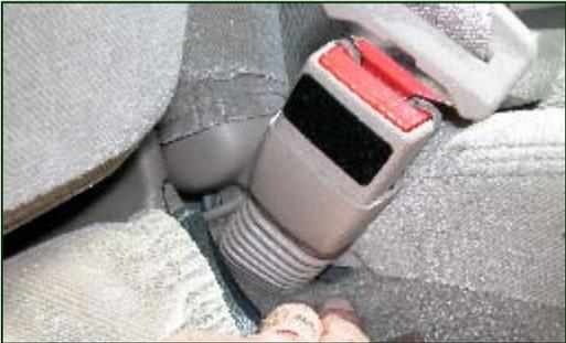
**Figure 10.** Fired driver's buckle pretensioner.
