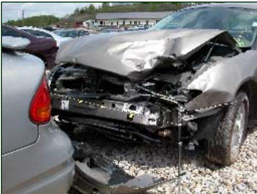
**Figure 5.** Frontal damage to the Ford Taurus.
