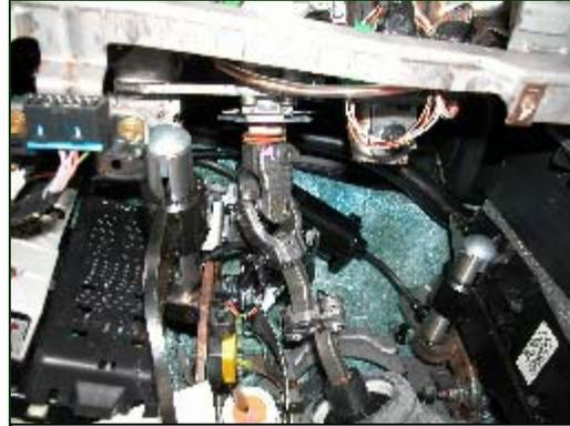
**Figure 3.** Adjustable pedal jackscrews.
