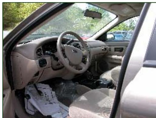
**Figure 12.** View of the non-deployed CAC frontal air bag system.
