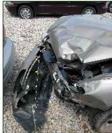
**Figure 6.** Lateral view documenting the depth of crush to the bumper beam.
