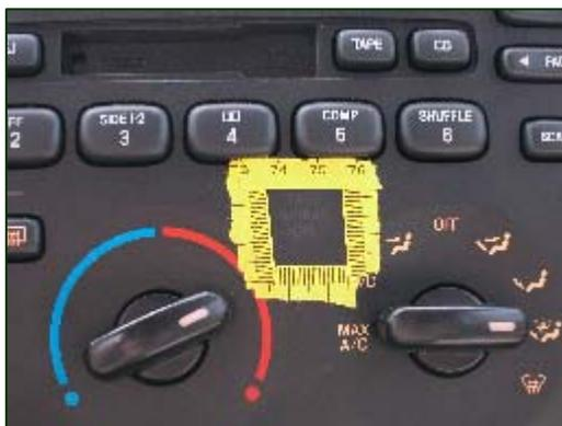
**Figure 11.** Passenger Air Bag ON/OFF status indicator lamp.
