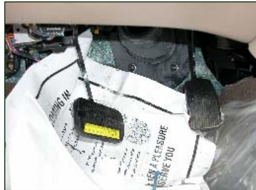
**Figure 8.** Deformed brake pedal from driver loading.
