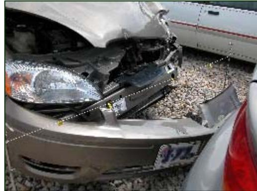
**Figure 7.** Green paint transfers from the dumpster impact.
