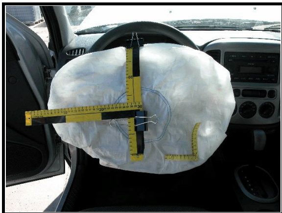
Figure 8. Driver's air bag. Contact to right lower quadrant.
