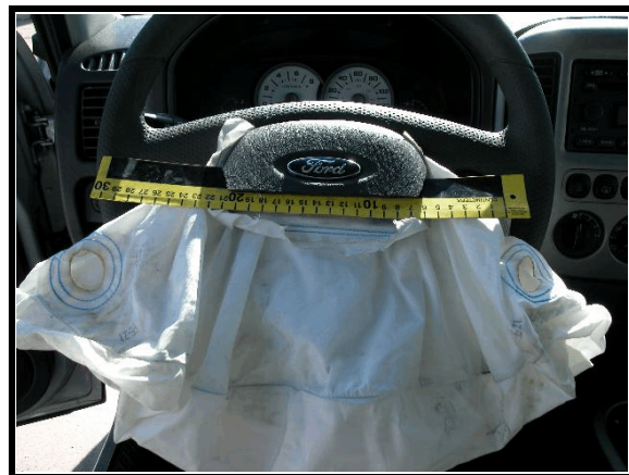
Figure 9. Driver's air bag. Scorched vent ports and top module cover.
