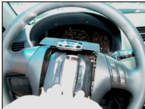
Figure 9. Close-up of secondary vinyl module flaps
