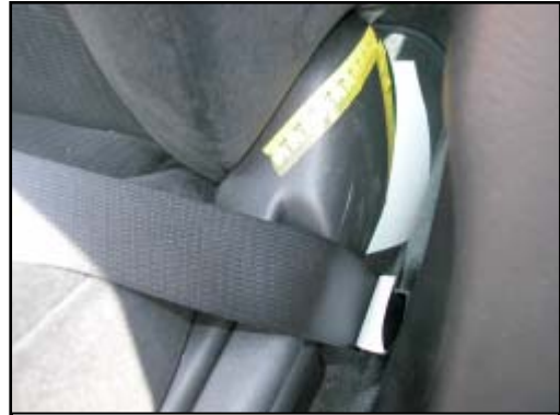
Figure 7. View of abrasion from driver's safety belt webbing
