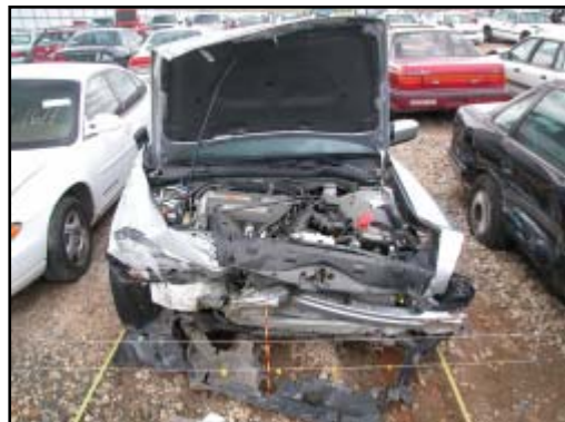
Figure 6. View of frontal damage showing end shift
