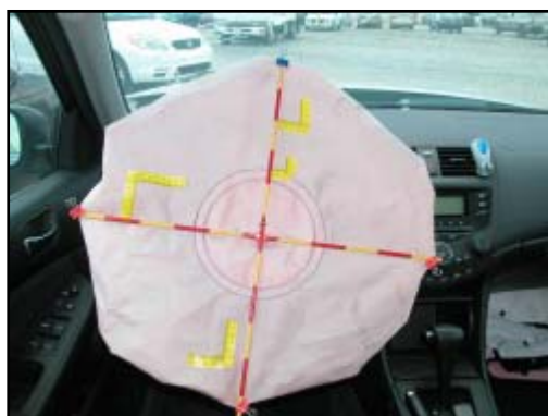
Figure 10. Deployed driver's air bag
