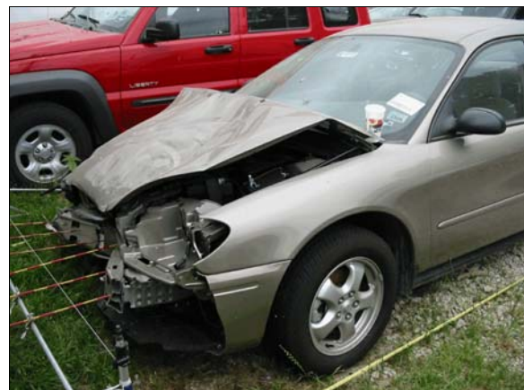
Figure 6: Left front view of front damage to case vehicle from crash attenuator impact, front bumper cover, grille and left headlamp/turn lamp assembly were missing (case photo #12)
