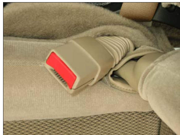
Figure 16: The driver's seat belt buckle showing compression of the buckle stalk due to the actuation of the pretensioner (case photo #37)
