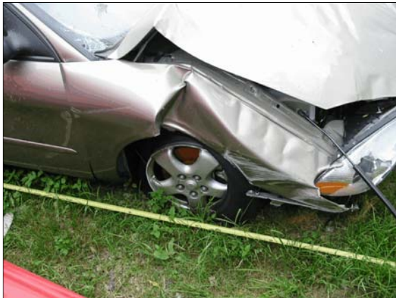
Figure 7: Damage to the right headlamp/turn lamp assembly, right fender and right front wheel from impact with the crash attenuator's cable assembly (case photo #19)
