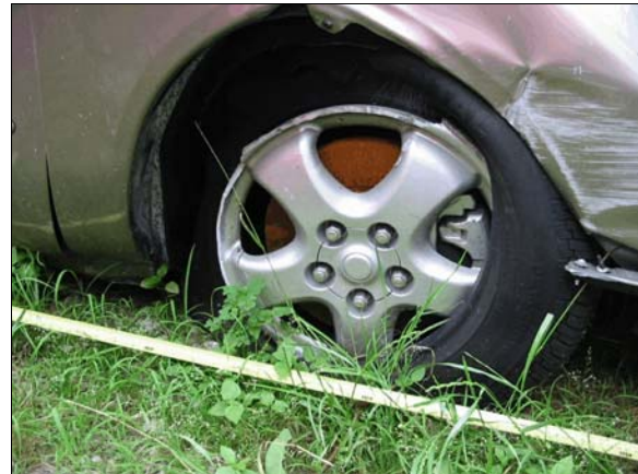
Figure 8: Close view of damage to case vehicle's right front wheel from crash attenuator's cable assembly (case photo #20)
