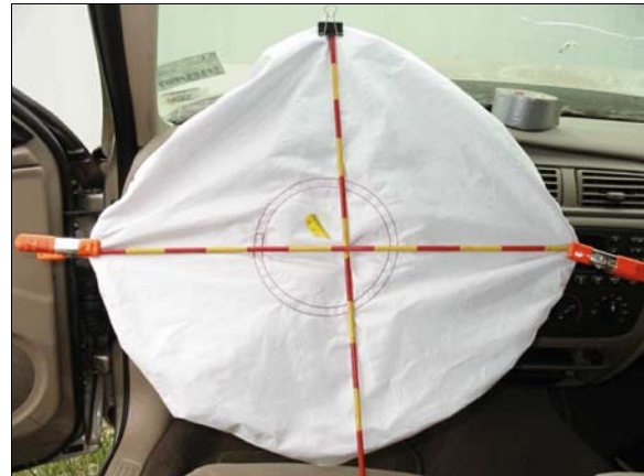
Figure 11: Overview of the driver's air bag, yellow tape shows location of yellow stain (case photo #28)
