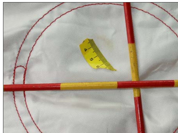
Figure 13: Close view of the yellow stain on the air bag to the right of the yellow tape (case photo #29)
