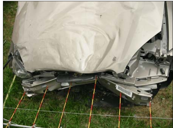
Figure 3: Damage to front of case vehicle from impact with crash attenuator; bumper cover, grille and left headlamp/turn lamp assembly were missing (case photo #10)
