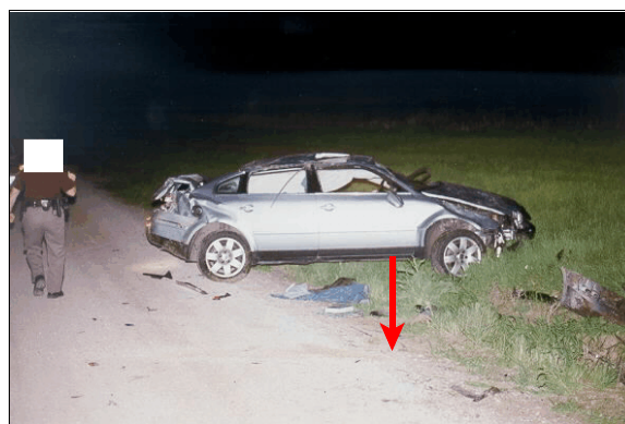
Figure 8: Police on-scene photo showing final rest position of case vehicle and damage to right fender and hood, arrow shows mark in gravel where right roof side rail impacted
