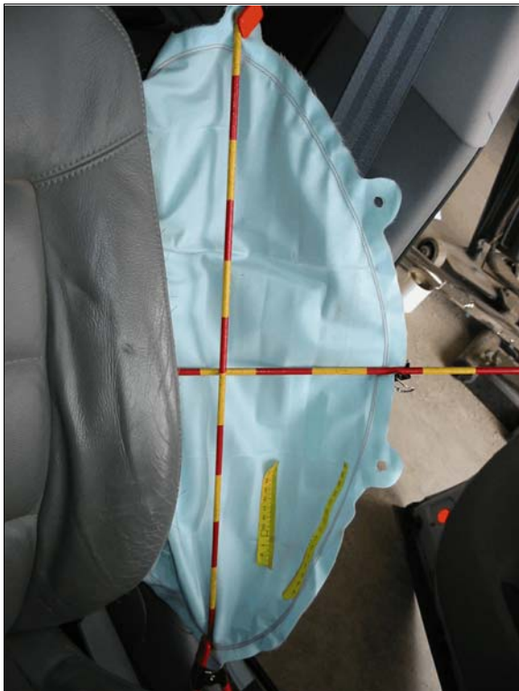
Figure 23: Inboard surface of case vehicle's driver seat back-mounted side impact air bag, yellow tape shows possible occupant contact
