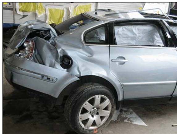
Figure 7: Damage to the back of case vehicle and right rear wheel
