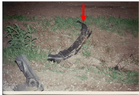
Figure 2: Police on-scene photo showing close view of ditch impact area; Note: components are case vehicle's lower front bumper fascia (arrow) and an unidentified undercarriage component
