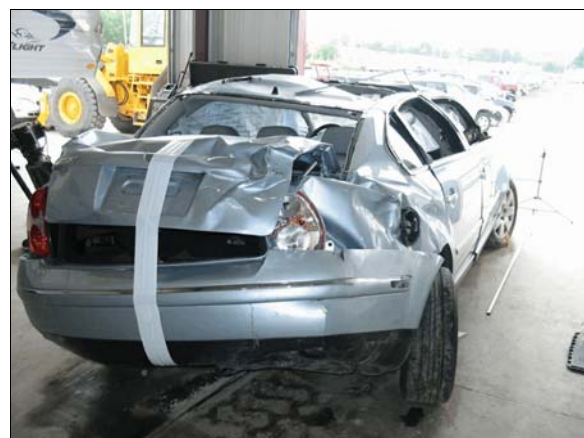
Figure 6: Damage to the back of the case vehicle
