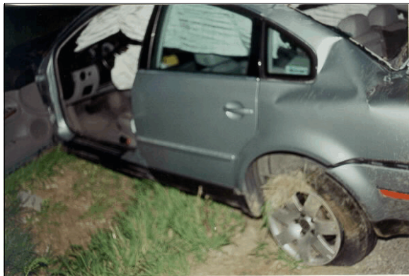
Figure 4: Police on-scene photo of the case vehicle at final rest showing dirt and grass jammed in rim and bead of left rear wheel
