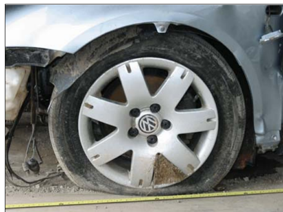
Figure 3: Damage and rearward displacement of case vehicle's left front wheel
