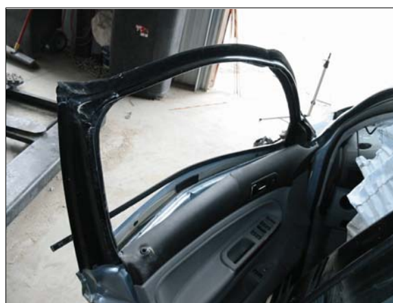
Figure 10: Case vehicle’s driver door is bowed outward from occupant loading
