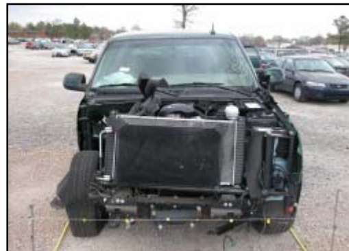
Figure 7. Overall view of the dismantled frontal damage.
