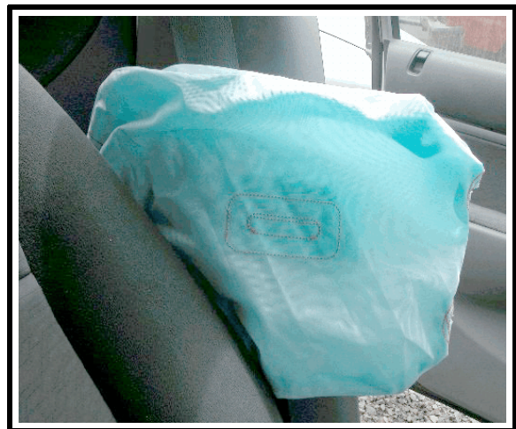
Figure 13. Driver's side seat back mounted side air bag—interior side
