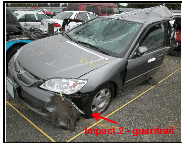
Figure 5. Front left, impact 2, guardrail
