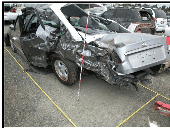
Figure 7. Left rear corner of case vehicle, impact 3 (tree)
