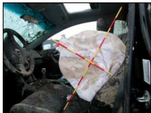
Figure 11. Close-up of deployed driver's side impact air bag
