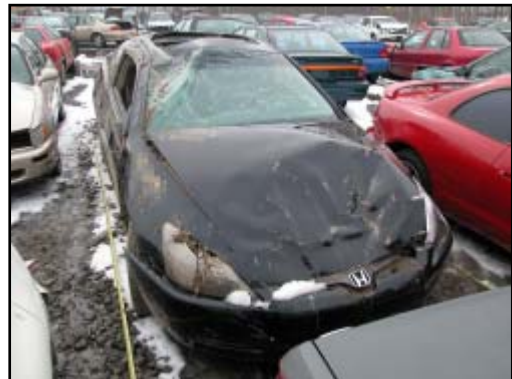
Figure 8. Overall view of rollover damage
