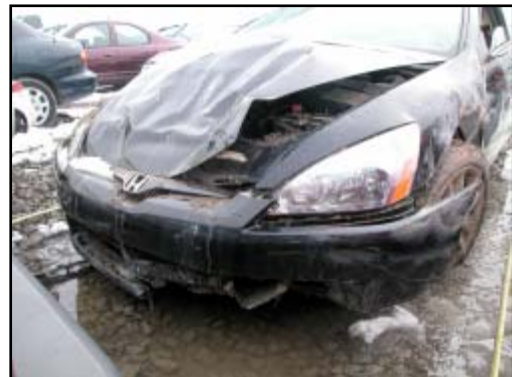
Figure 6. View showing damage to the front left area of the undercarriage beneath the bumper
