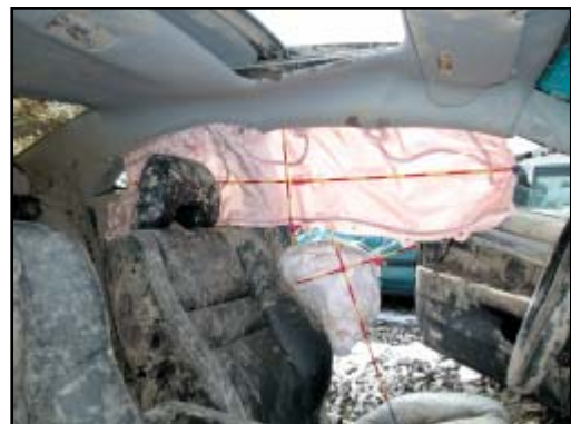
Figure 10. Overall view of the driver's side impact air bag and left side IC
