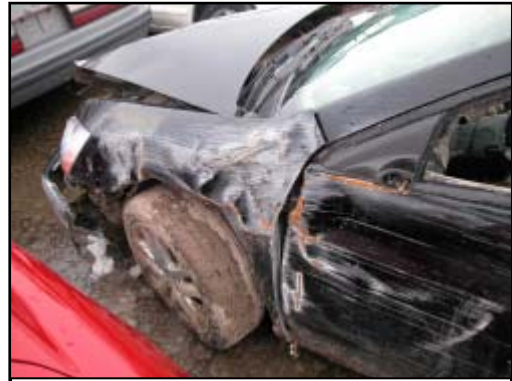
Figure 7. View of left side abrasions and damage to the left front fender
