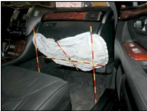
Figure 12. Deployed front right passenger's knee air bag in deployed position
