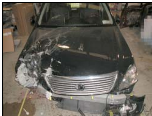
Figure 4. Overhead view of frontal damage and hood contact
