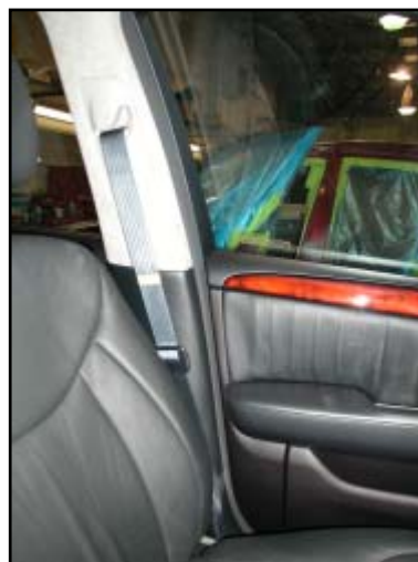
Figure 6. View of restricted driver's safety belt
