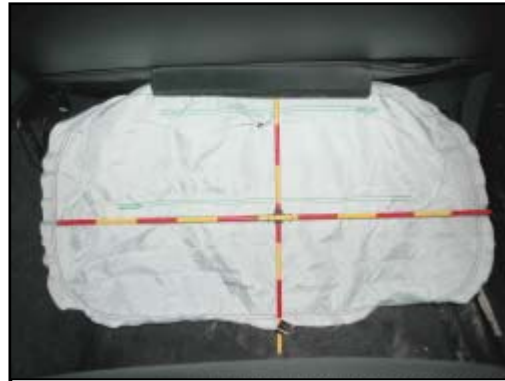
Figure 13. Rear aspect (against instrument panel) of deployed front right passenger's knee air bag
