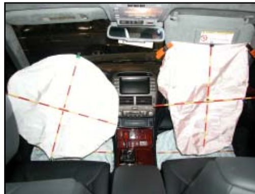
Figure 10. View of deployed frontal air bags and deployed knee air bags
