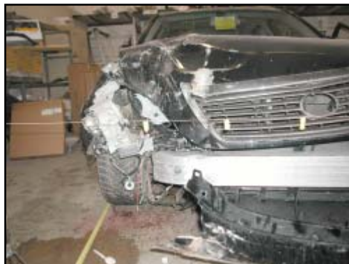
Figure 5. Close up of front right damage from the mailbox post
