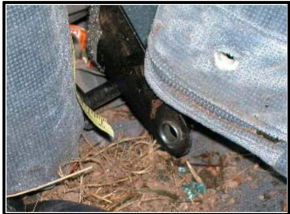
Figure 10. View of the bottom of the right rear seat back, the center arm rest, and the pin and pin hole
