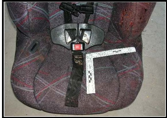
Figure 27. Seat from case vehicle, upper thigh straps not in place
