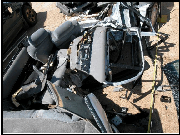
Figure 20. Overhead view of side damage as seen from the rear of the vehicle (1997 Buick LeSabre)
