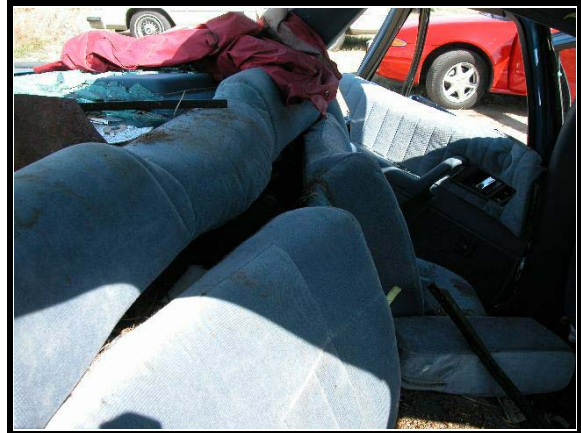
Figure 11. Overview of rear seat failure/intrusion
