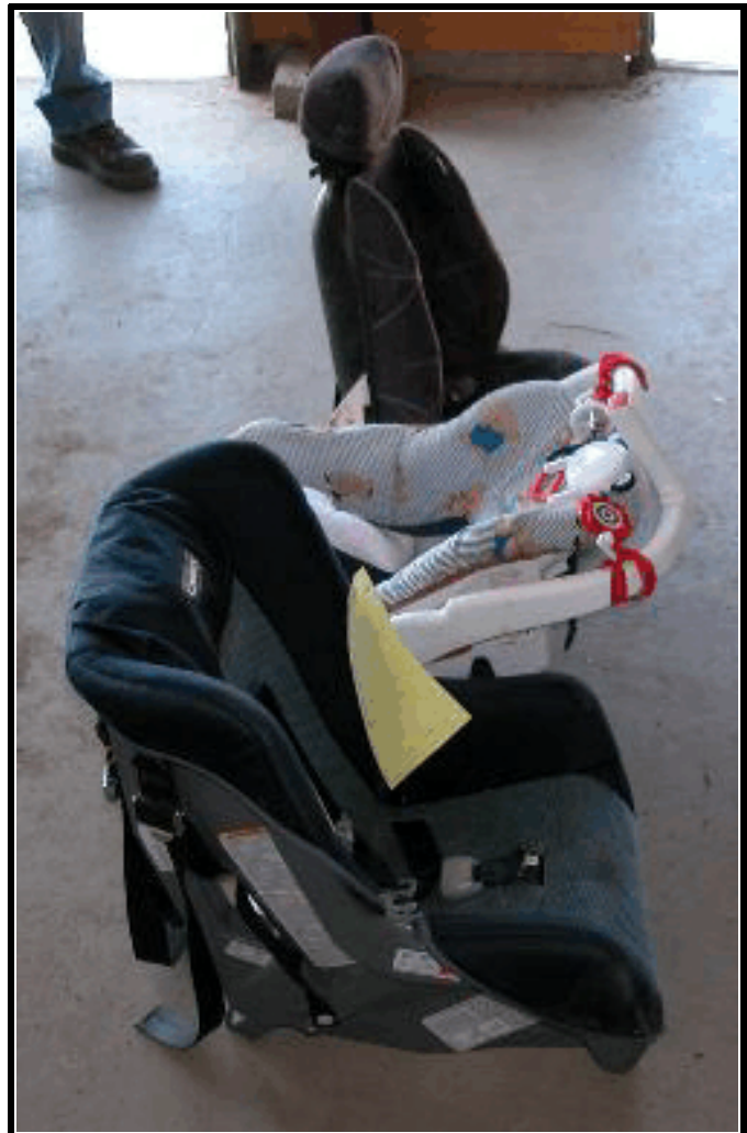
Figure 3. Child seat configuration in rear seat. Front of vehicle to the right. From top to bottom, Century Breverra Premier booster seat, Evenflo Discovery infant safety seat, Century 1000 STE convertible safety seat.
