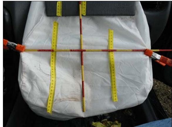
Figure 12: Case vehicle's front right passenger air bag, yellow tape outlines area of skin transfer on air bag and module cover flap and possible cloth transfer on air bag
