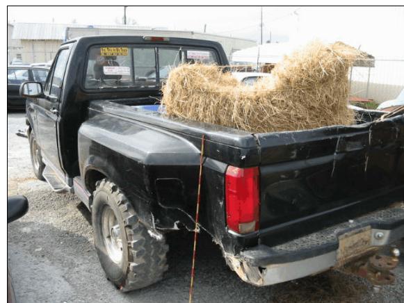
Figure 14: Overview of damage to left rear side of Ford from impact with the case vehicle
