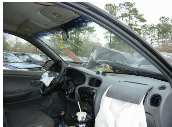
Figure 10: Overview of location of front right air bag and case vehicle’s instrument panel, windshield and steering wheel
