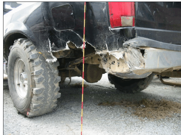
Figure 4: Damage to left rear side of Ford's truck bed from impact with the case vehicle
