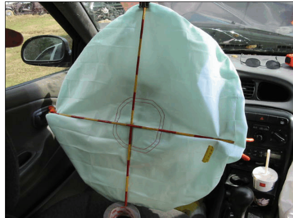
Figure 9: Overview of case vehicle’s driver air bag, yellow tape shows light scuff on air bag, which appeared related to deployment
