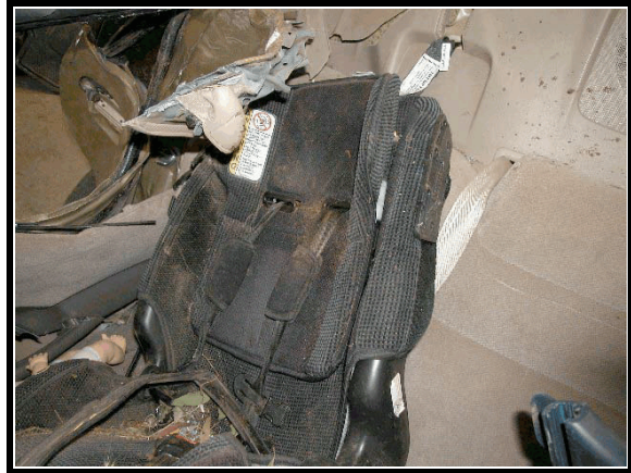
Figure 17. Child seat with view of intruding C pillar and splatter pattern to right of image
