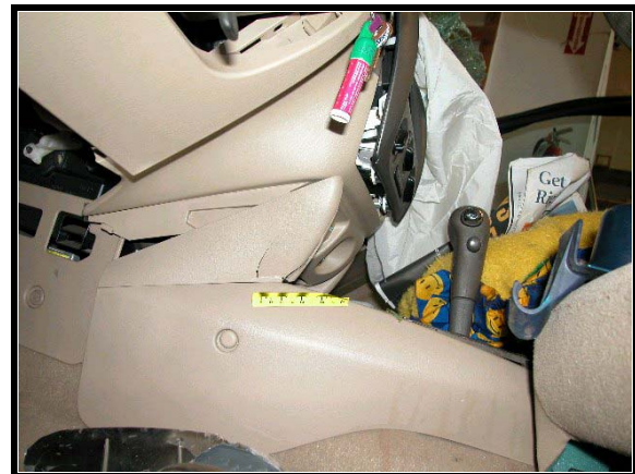
Figure 15. Driver contact to lower center console
