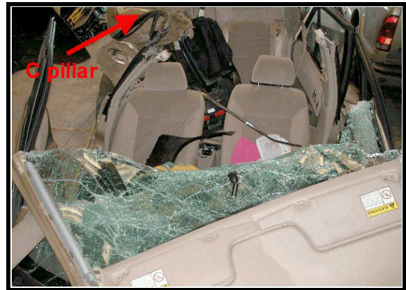
Figure 10. Overview of right side intrusion
