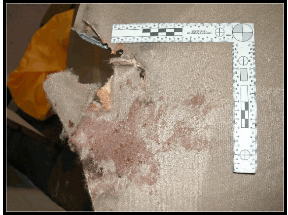
Figure 16. Head contact to right C pillar/roof transition
