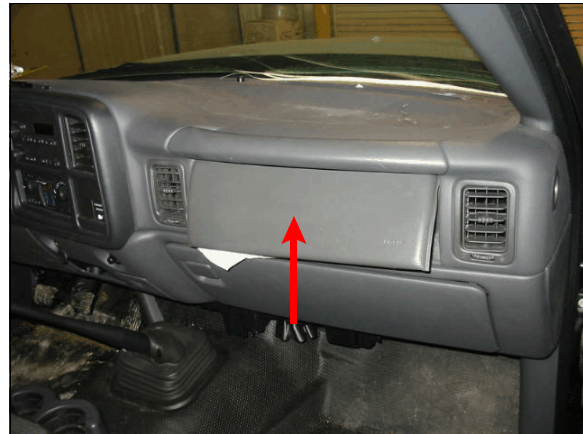
Figure 10: Overview of front right air bag module flap, indicated by arrow (case photo #38)
