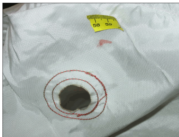
Figure 12: Vent port of left side of front right passenger air bag and blood stain (case photo #36)
