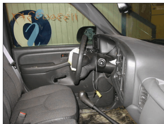
Figure 6: Case vehicle’s steering assembly viewed from right showing deformation to upper portion of rim (case photo #28)
