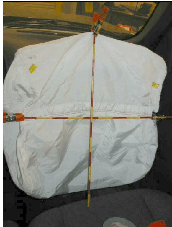
Figure 11: Front right passenger air bag. Yellow tape shows location of blood stains (case photo #33)
