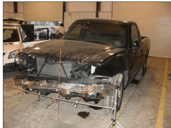
Figure 3: Oblique view of front and left sides of case vehicle showing direct damage to the front, each stripe on rods is 5 cm (2 in), (case photo #08)
