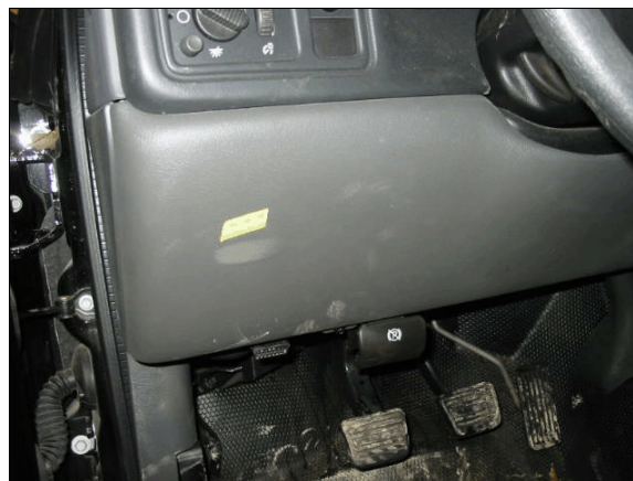
Figure 7: Tape shows scuff on driver's left knee bolster (case photo #29)
