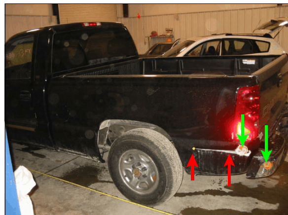
Figure 4: Damage to left quarter panel from impacts with concrete median barrier (green arrows) and guardrail [red arrows (case photo #11)]
