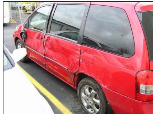
Figure 3. Continuation of the sideswipe damage to the Mazda.
