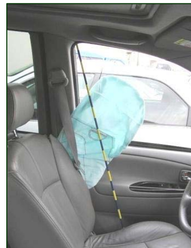
Figure 6. Deployed side impact air bag.
