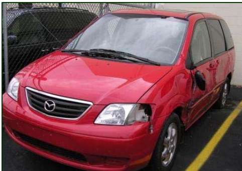
Figure 2. Left sideswipe damage to the Mazda MPV.
