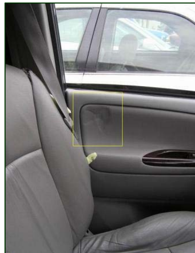
Figure 9. Driver contact to the left door panel.
