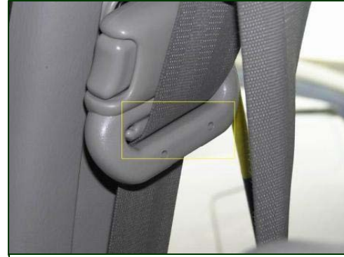
Figure 7. D-ring frictional transfer.
