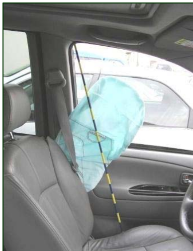
Figure 8. Deployed side impact air bag.
