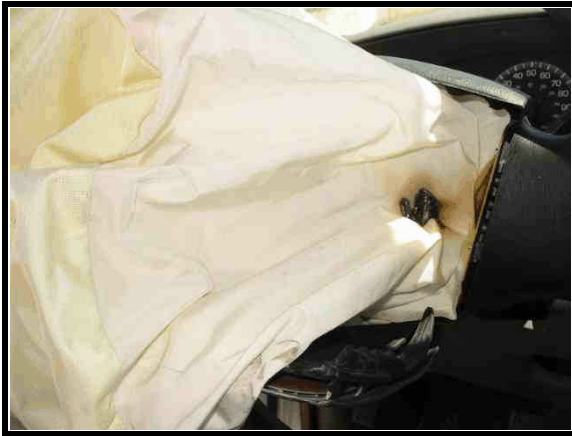
Figure 11. Burn to right side of driver's air bag
