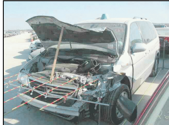
Figure 3: Case vehicle's front and left side, above-bumper crush profile
