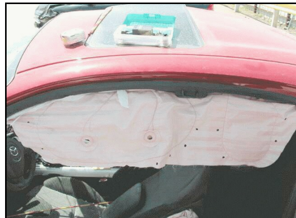
Figure 10: Exterior view, whole left side inflatable curtain air bag
