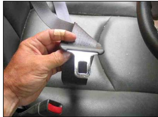
Figure 7 - Front left safety belt latch plate.
