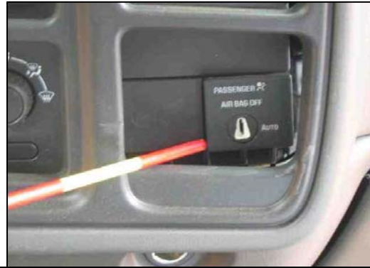
Figure 8 - Air bag cutoff switch.
