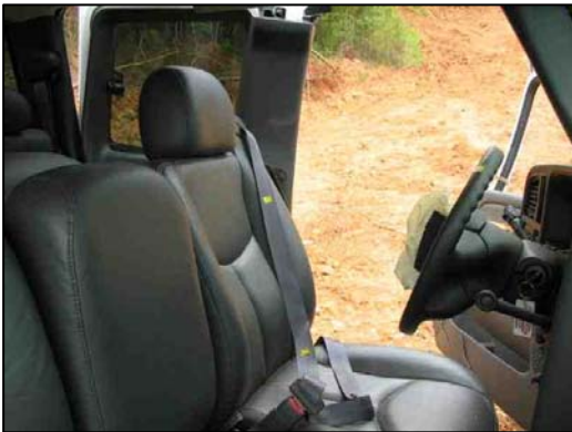
Figure 6 - Loaded front left seat belt and deformed steering wheel rim.
