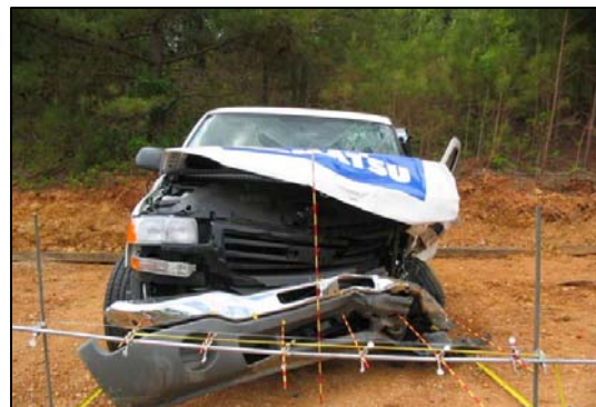
Figure 4 - 2004 GMC Sierra crush profile.
