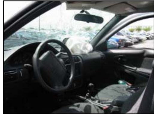
Figure 10. View of the non-deployed driver's air bag and the deployed front right air bag.
