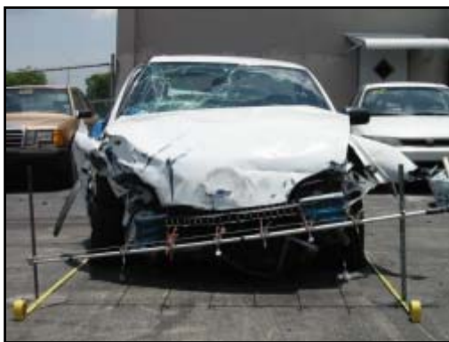
Figure 8. Frontal damage from the initial impact with the Jaguar.
