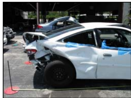
Figure 9. Right side damage from the secondary impact with the Jaguar. Damage was overlapped by a rear impact.
