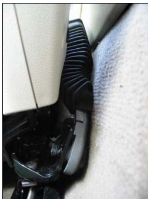
Figure 14. Fired driver's safety belt pretensioner.
