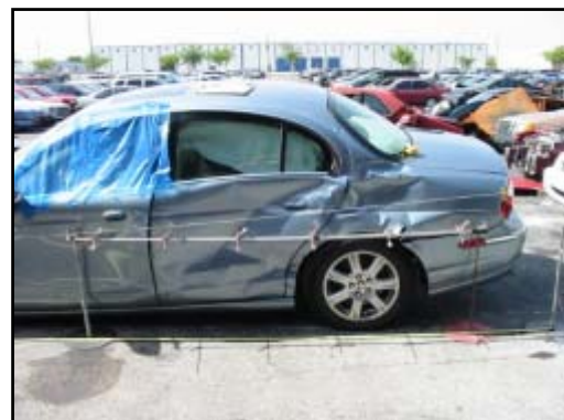
Figure 6. Left side damage from the secondary impact with the Chevrolet.
