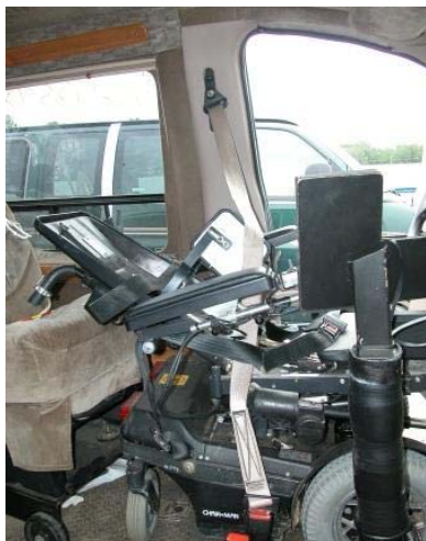
Figure 15. Routed positions of the manual safety belts.
