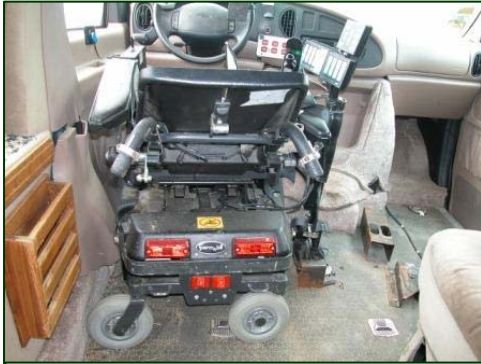
Figure 6. Motorized wheelchair secured into the EZ-Lock restraint device.
