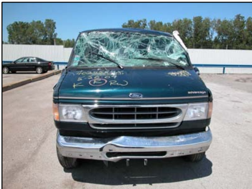
Figure 10 – Frontal damage to the 1998 Ford E-150
