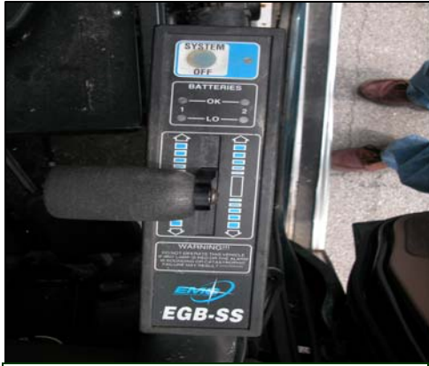
Figure 3. Adaptive hand control for throttle and brake functions.
