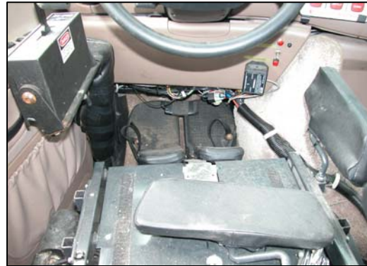
Figure 17. Wheelchair footrests inadvertently positioned behind and under the brake pedal.
