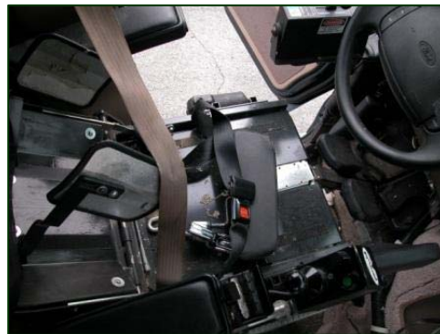
Figure 16. Wear mark of the shoulder belt webbing from chest stabilizer.
