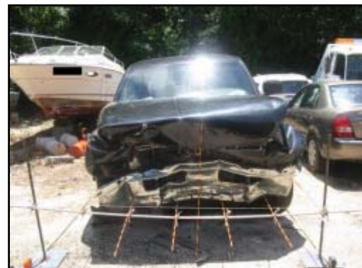
Figure 7. Crush profile for the 1999 Dodge Ram.
