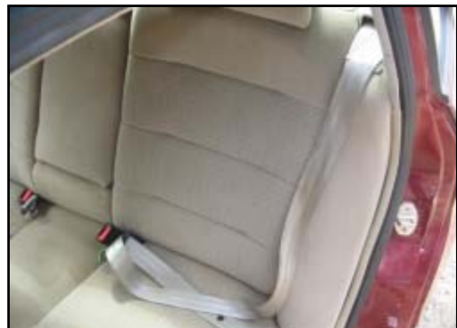
Figure 9. Rear left safety belt with fired pretensioner.
