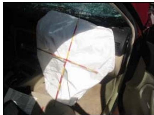
Figure 14. Deployed front right air bag.
