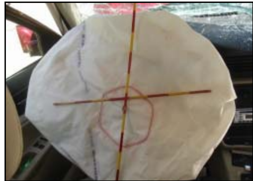
Figure 13. Deployed driver's frontal air bag.
