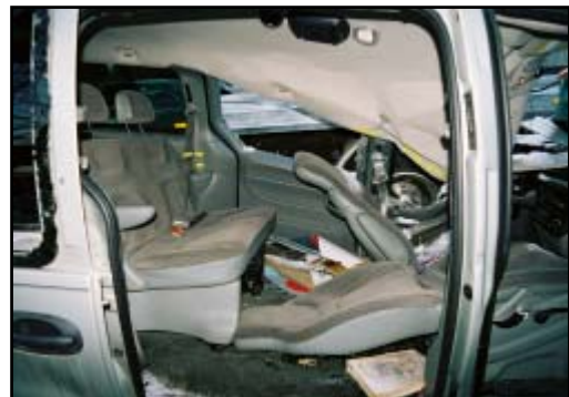
Figure 7. View from right side showing intrusions into front and second row seat positions
