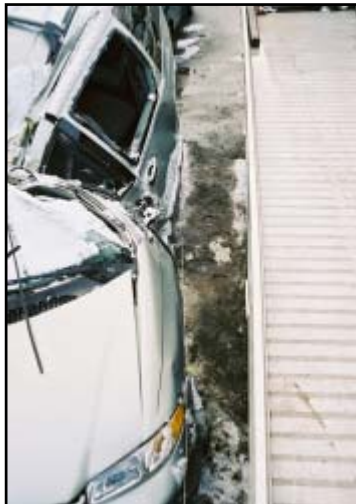
Figure 5. View of left side damage to the Grand Caravan
