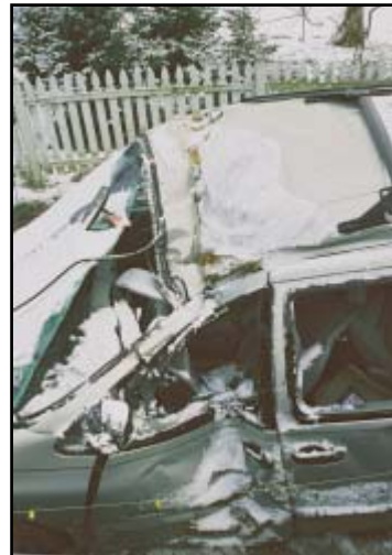
Figure 6. Close-up of direct damage from the tree
