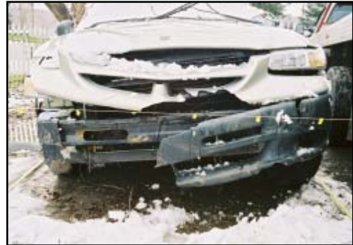
Figure 4. Close up of frontal damage to the Grand Caravan
