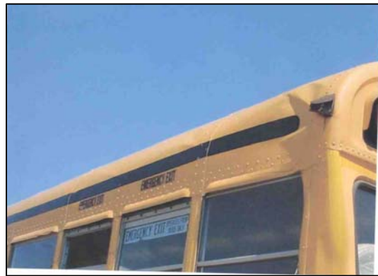
Figure 7 - Damage to the left rear of 1993 Blue Bird 3800.
