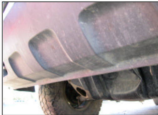
Figure 5. Damage to stone guard from pond.
