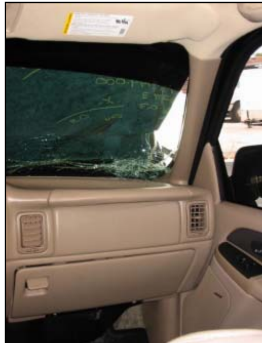
Figure 8. Non-deployed front right air bag.
