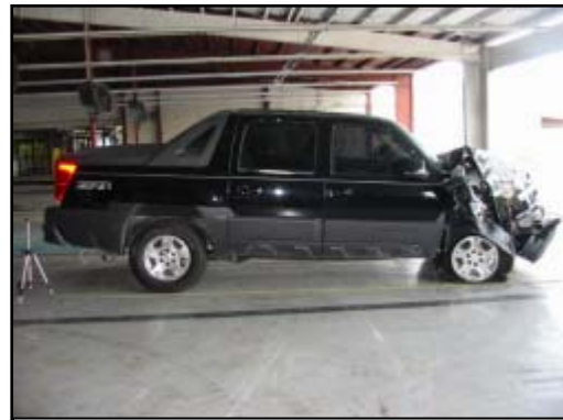
Figure 6. Lateral view of the crush profile.
