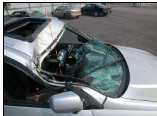
Figure 8. Lateral view showing direct damage from the tree
