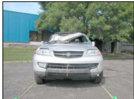
Figure 6. Frontal view showing minor lower bumper fascia damage
