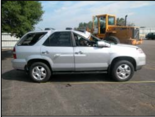
Figure 9. Left side view of the damaged MDX
