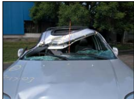
Figure 7. Frontal view of green house damage to the MDX
