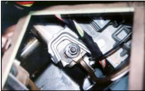
Figure 10. Left shear bracket displacement of the Sable.
