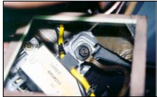
Figure 11. Right shear bracket displacement of the Sable.
