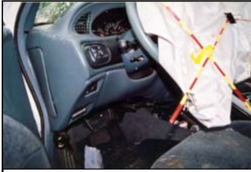
Figure 8. View of intrusion to the Sable's side panel forward of A-pillar.
