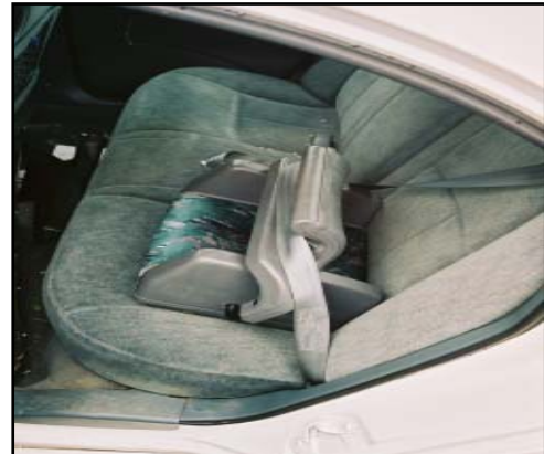
Figure 14. CSS found in rear left position at inspection.
