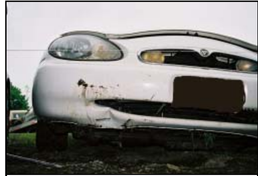
Figure 6. Damage to Sable from Embankment.
