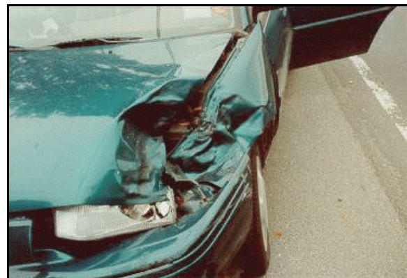
Figure 3: Case vehicle's direct damage at front left corner (case photo #11)
