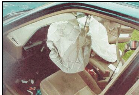
Figure 4: Driver's air bag and automatic shoulder belt (case photo #16)
