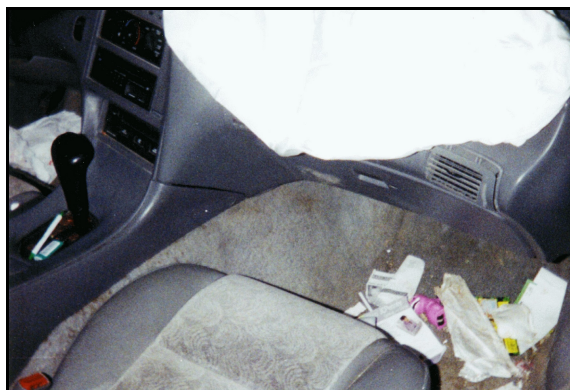
Figure 5: Front right seat area and partial view of front right passenger's air bag (case photo #14)
