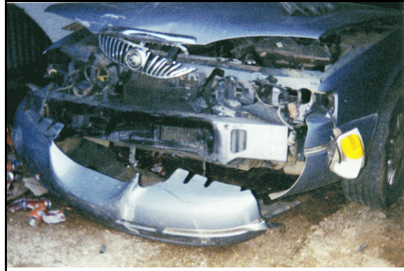
Figure 3: Front-left view of case vehicle's frontal damage (case photo #05)
