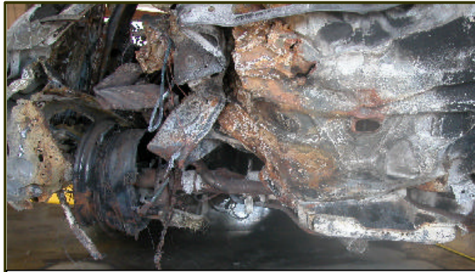
Figure 18. Separated filler tube and left rear quarter panel at lower left corner of image.
