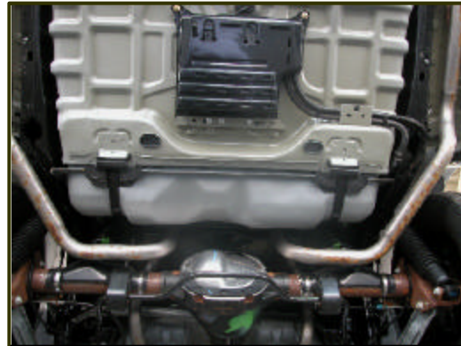
Figure 12. Undercarriage view of an exemplar 2003 CVPI depicting the fuel system and shield kit.
