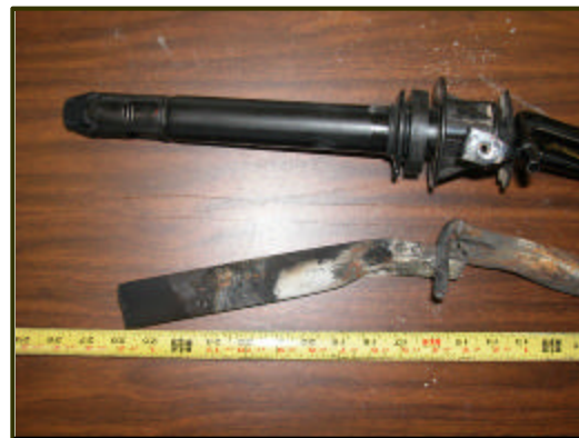
Figure 20. Close-up view of the separation location of the filler tube.
