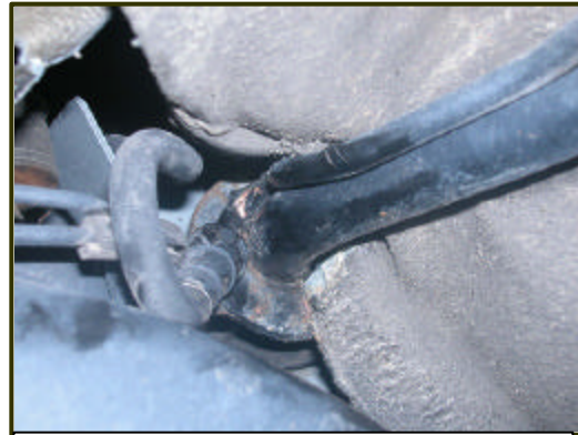
Figure 22. Deformation of the filler tube and inner fender edge from engagement during crash.
