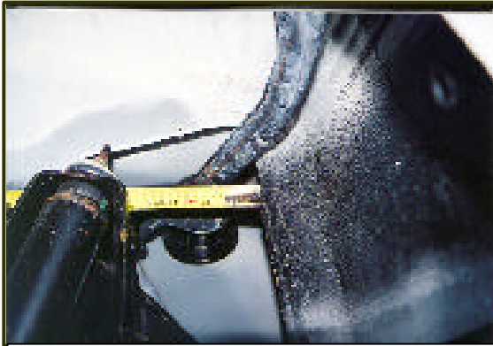
Figure 16. Filler tube position in relation to the inner fender on an exemplar 2003 CVPI.
