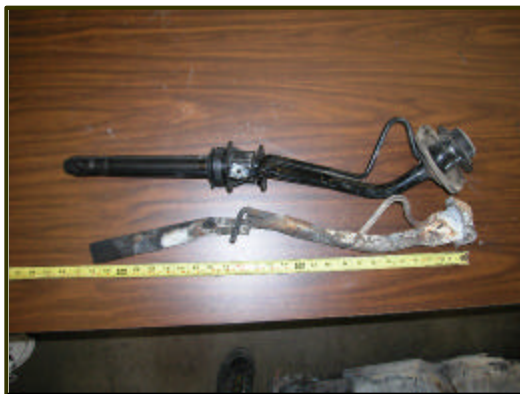
Figure 19. The damaged and separated filler tube in relation to an exemplar tube.
