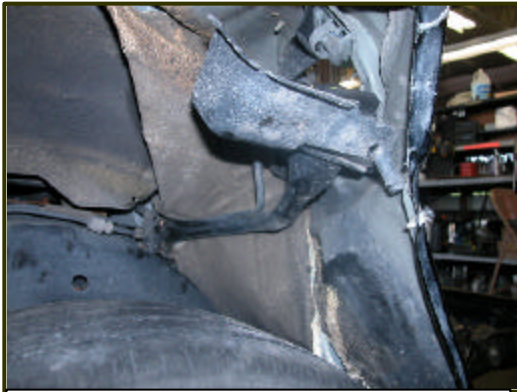
Figure 21. Filler tube location on the 1999 Lincoln Town Car.
