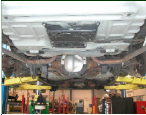
Figure 13. Shield kit installed on an exemplar Crown Victoria.
