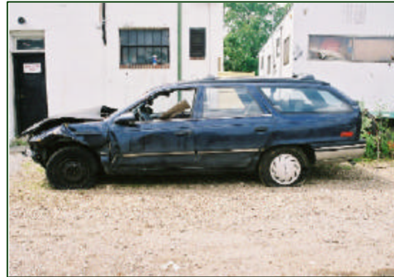
Figure 11. Lateral view documenting the extent of the frontal crush.
