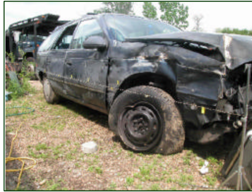
Figure 9. Right side damage to the Ford Taurus.
