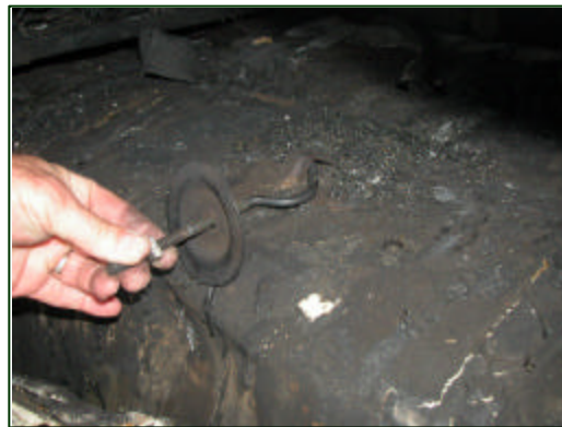
Figure 20. Spare tire hold-down bracket and anchor loop.
