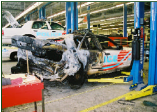
Figure 1. Right rear view of the crush pattern and resultant fire damage to the 2000 Ford Crown Victoria.
