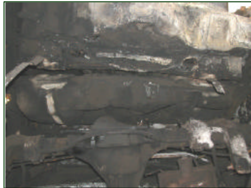
Figure 16. Deformed fuel tank prior to removal
