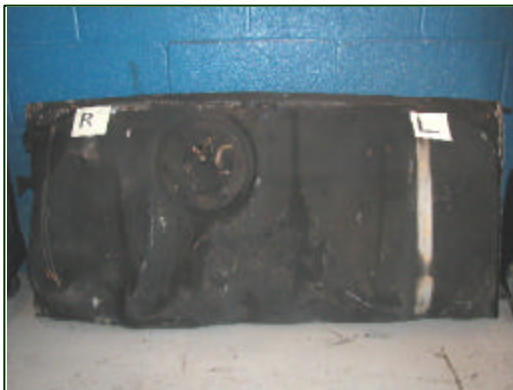
Figure 17. Forward aspect of the removed fuel tank.
