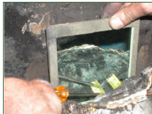
Figure 22. Crease to the back wall of the trunk from washer engagement.
