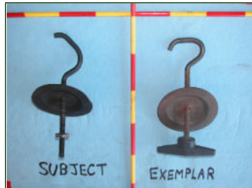
Figure 21. Subject vehicle hold-down bracket compared to an exemplar
