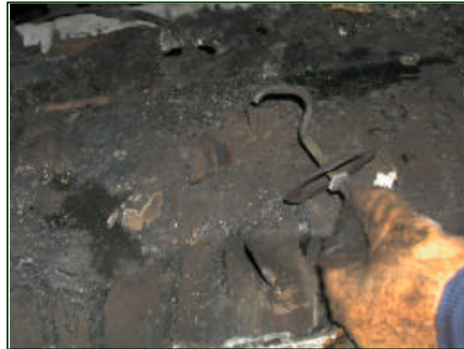
Figure 25. Loading, elongation, and separation of the bracket from the anchor loop.
