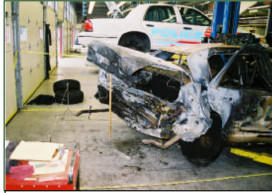
Figure 6. Lateral view documenting the extent of crush to the back plane.
