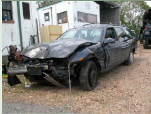
Figure 10. Frontal view of the resultant damage from the Crown Victoria impact.
