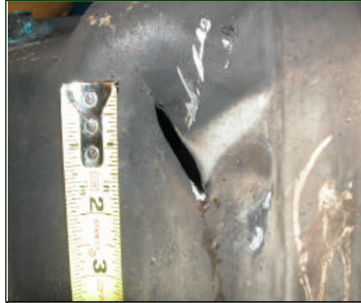
Figure 19. Puncture to the upper aspect of the fuel tank with adjacent burn.
