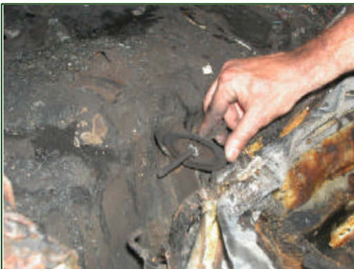
Figure 26. CW rotation of the bracket and engagement against the trunk wall.
