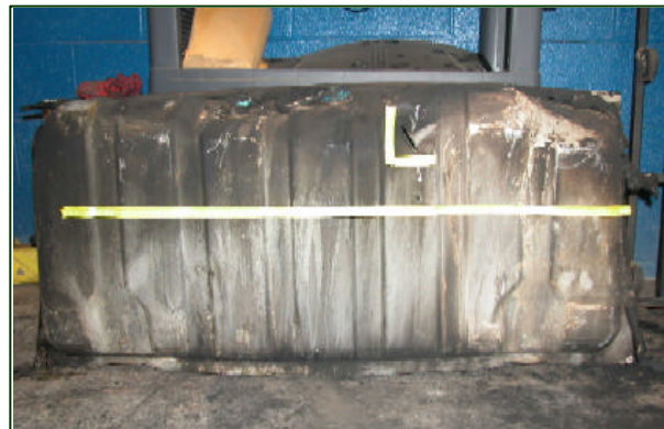
Figure 18. Rear aspect of the fuel tank with puncture outline with calibrated tape.
