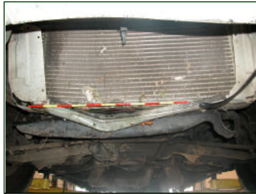
Figure 8. Lower radiator support impact damage.
