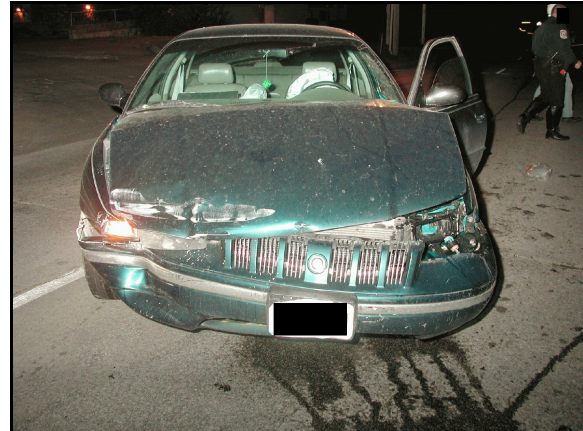
Figure 2: Front of case vehicle at final rest, showing moderate frontal damage (case photo #08)
