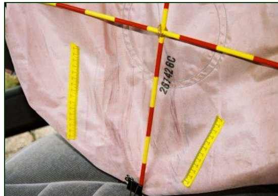
Figure 9. Fabric transfers to the lower face of the driver's air bag.
