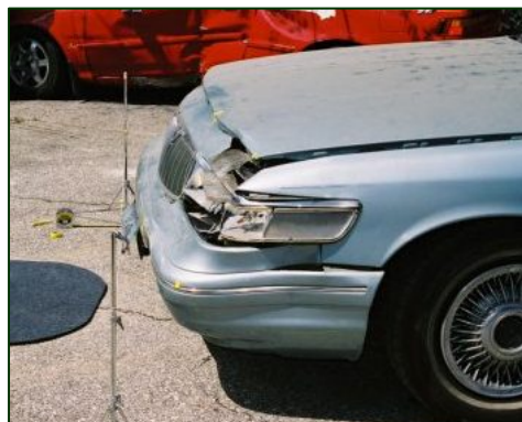
Figure 6. Lateral view of the crush depth.
