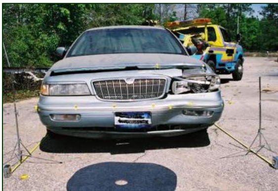
Figure 5. Front left damage to the Grand Marquis.
