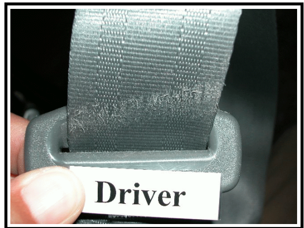
Figure 21. Loading to driver's seat belt
