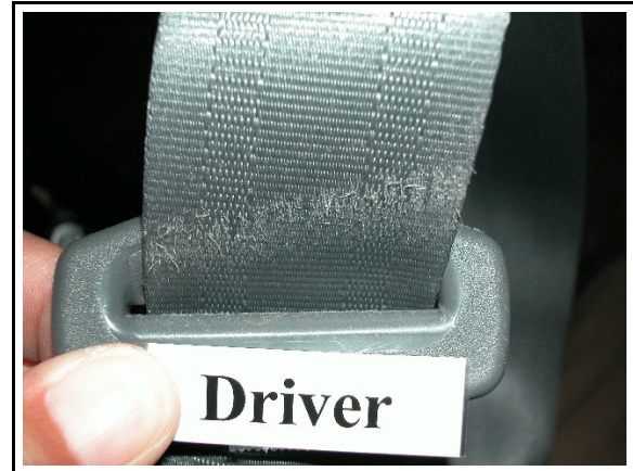
Figure 8. Loading marks to driver's seat belt
