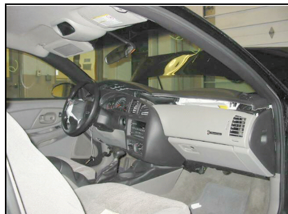
Figure 6: Active instrument panel raised across entire width (case photo #32)
