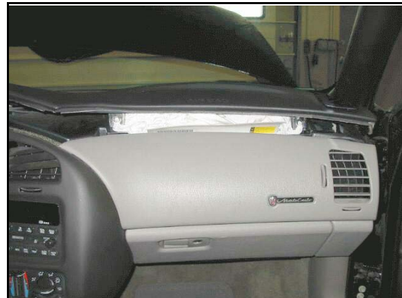
Figure 5: Raised top of active instrument panel, showing the opening through which the front right air bag deployed (case photo #41)
