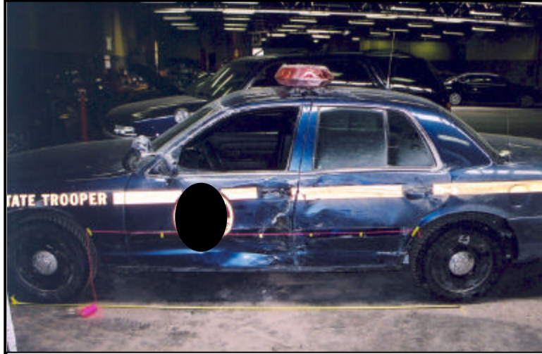
Figure 6: Left side view of the damaged Ford.
