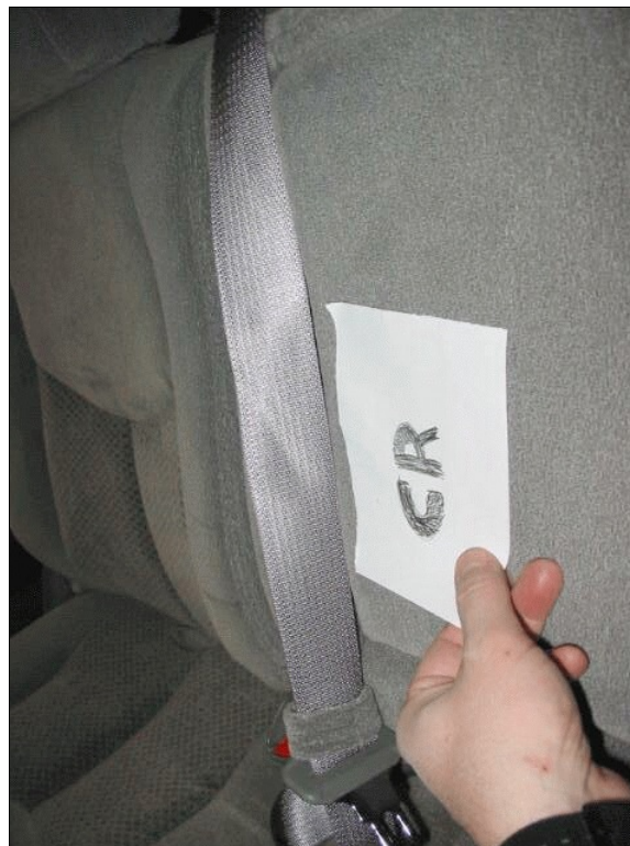
Figure 23: Seat belt webbing for case vehicle's back center passenger showing stress marks indicative of restraint usage (case photo #54)
