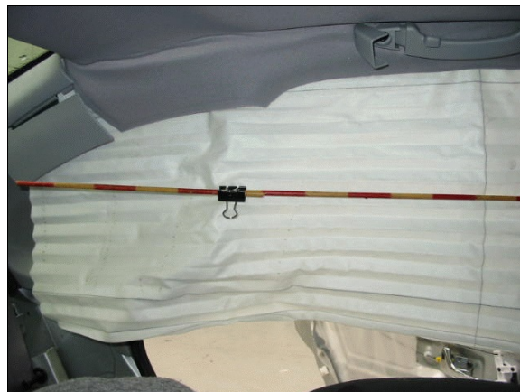
Figure 31: Inboard surface of Volvo’s left side inflatable curtain protecting back left seating area; Note: no apparent evidence of occupant contact (case photo #89)
