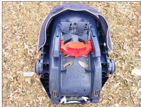
Figure 19: Overhead view of underneath side of shell of infant child safety seat used by case vehicle's back center passenger; Note: no apparent damage (case photo #105)
