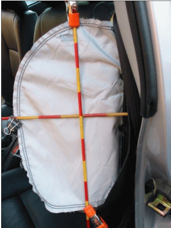
Figure 26: Outboard surface of Volvo's driver seat back-mounted side impact air bag showing no evidence of intrusion or contact (case photo #82)
