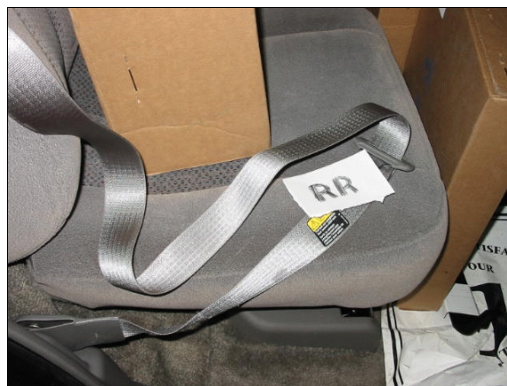
Figure 24: Seat belt webbing for case vehicle's back right passenger showing stress marks indicative of occupant loading (case photo #48)
