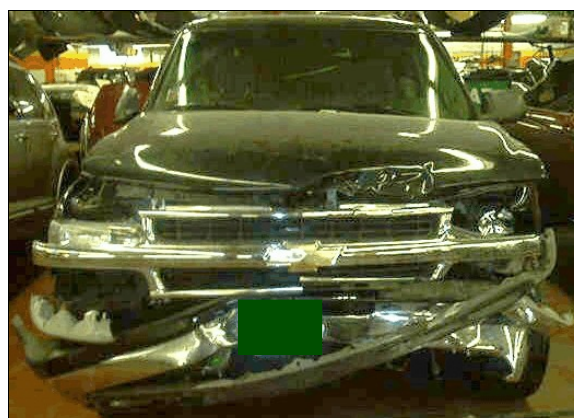
Figure 5: Body shop photo of case vehicle's frontal damage showing damage across entire front (case photo #108)
