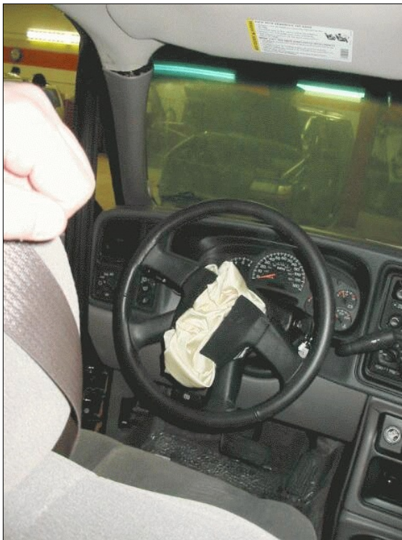
Figure 9: Case vehicle’s driver seating area showing no apparent evidence of occupant contact to the steering wheel, instrument panel, or green-house components (case photo #23)
