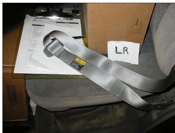
Figure 22: Seat belt webbing for case vehicle's back left passenger showing a wavy pattern indicative of occupant loading (case photo #51)
