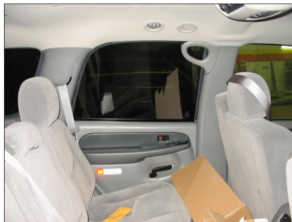
Figure 11: Case vehicle's second seating area showing no apparent contact evidence to the driver's seat back, interior surface of the left rear door, or greenhouse components (case photo #58)
