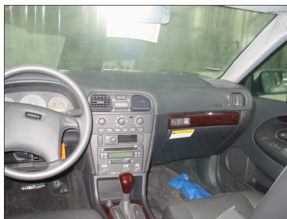
Figure 25: Volvo's front seating area showing non-deployed driver and front right passenger air bags; Note: steering wheel, instrument panel, and greenhouse area show no apparent evidence of occupant contact (case photo #70a)
