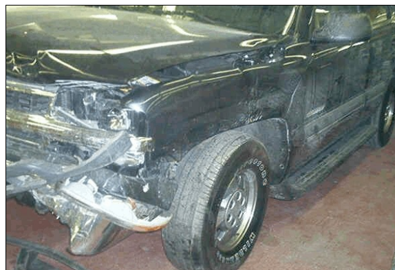
Figure 6: Body shop photo showing case vehicle's front left direct damage and induced damage to left fender and left front door (case photo #111)
