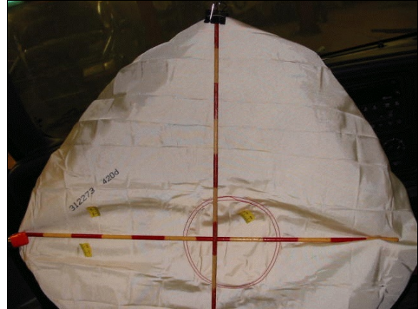
Figure 13: Case vehicle's deployed driver air bag showing makeup smear within center circular stitching and possible contacts toward 9 o'clock position (case photo #29)
