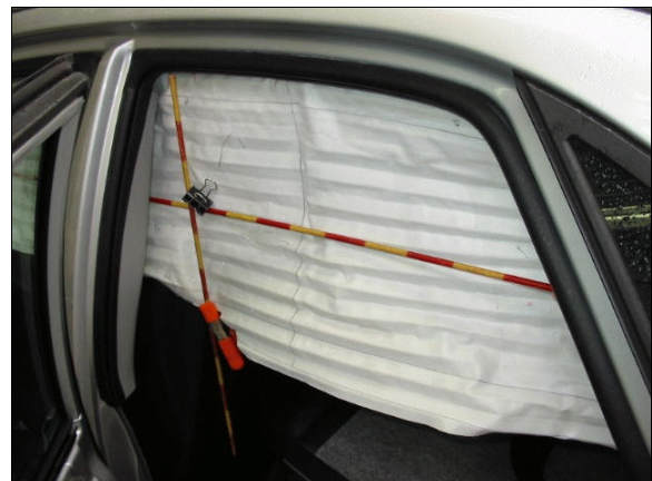
Figure 29: Outboard surface of Volvo's left side inflatable curtain protecting back left seating area (case photo #91)
