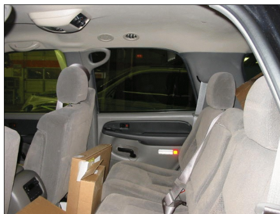
Figure 12: Case vehicle's second seating area showing no apparent occupant contact evidence to the front right passenger's seat back, interior surface of the right rear door, or greenhouse components (case photo #59)
