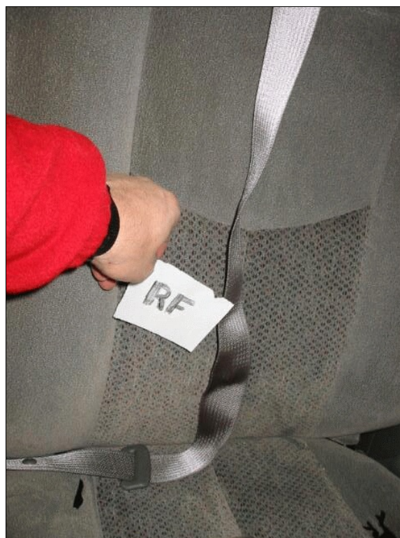
Figure 21: Safety belt webbing for case vehicle's front right passenger showing a wavy pattern indicative of occupant loading (case photo #17)
