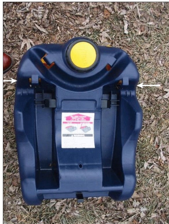
Figure 15: Overhead view of infant child safety seat's detachable base; arrows indicate where case vehicle's safety belts attach through slots in base (case photo #101)
