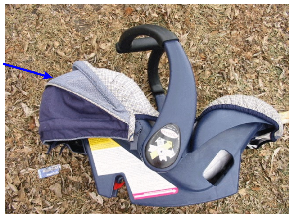
Figure 18: Overhead view of left side of infant child seat used by case vehicle's back center passenger showing warning label and red and white leveling arrow at bottom of label; Note: child's head is positioned toward arrow (case photo #104)
