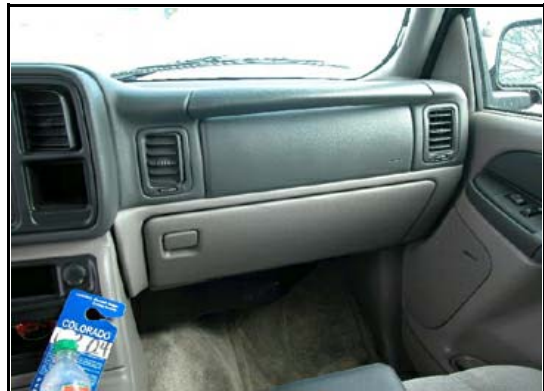
Figure 4. Not deployed front right passenger's air bag
