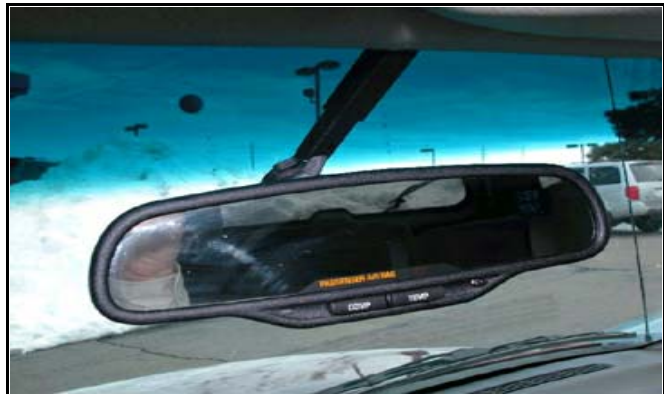
Figure 6. Passenger Sensing System monitored on rear view mirror
