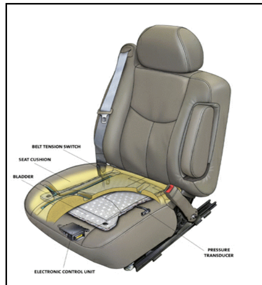
Figure 5. Front right Passenger Sensing System
