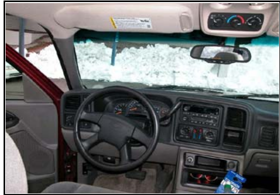
Figure 3. Not deployed driver's air bag
