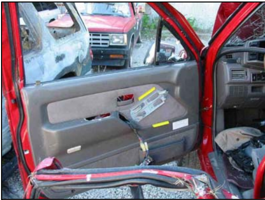
Figure 15 - Contact evidence on front left door panel.
