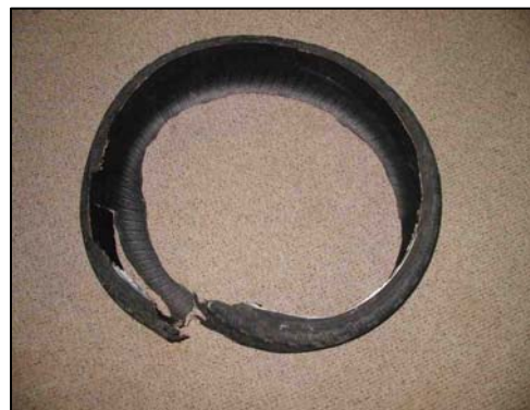
Figure 13 - View of post-crash right rear tread.
