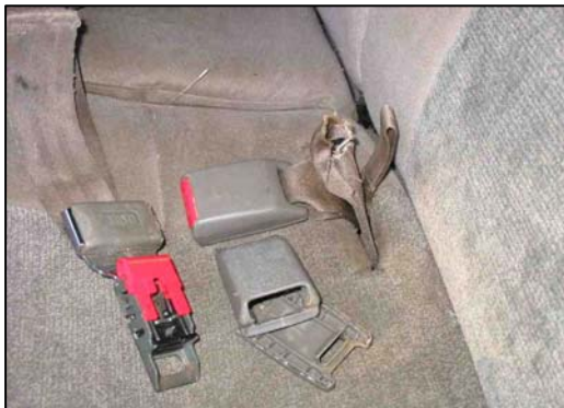
Figure 17 - Post-crash condition of center lap belt.
