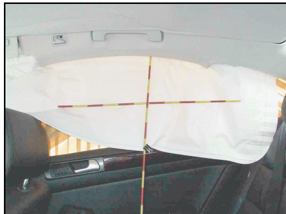
Figure 13: Back seat portion of right curtain wall
