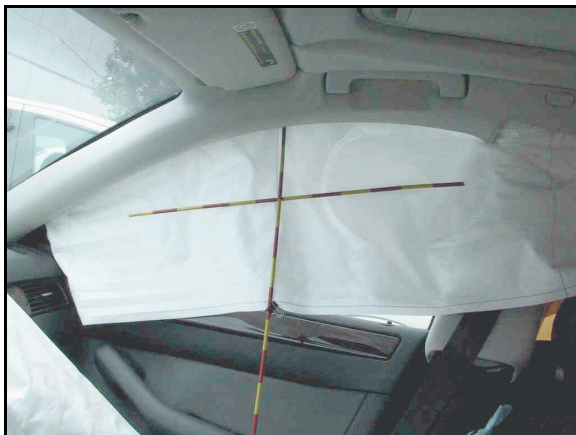
Figure 12: Front seat portion of right curtain wall
