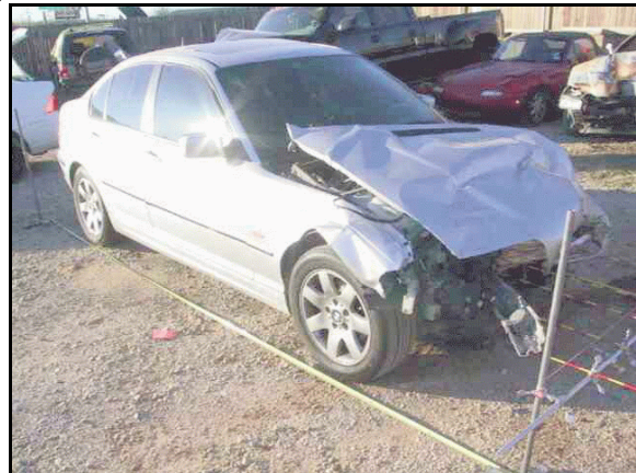
Figure 3: Case vehicle's front and right; note, overlapping damage from two impacts on the front
