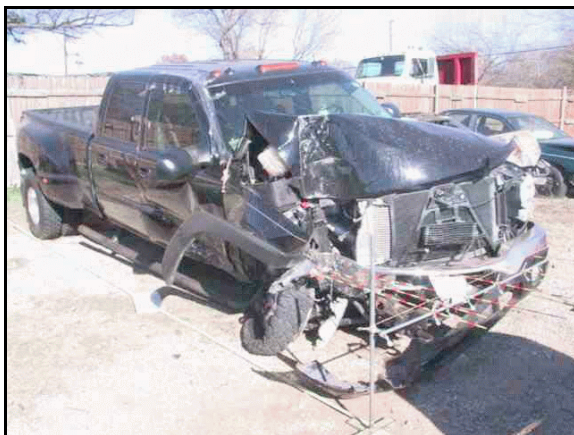
Figure 16: Other vehicle, showing overlapping damage at front right corner area
