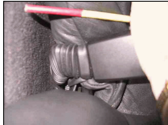
Figure 15: Passenger' s actuated pretensioner; note, buckle stalk deformed; see also Figure 14
