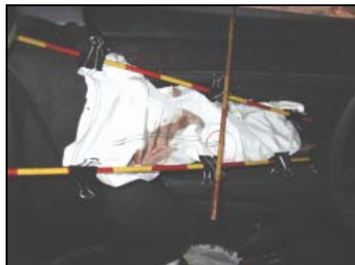
Figure 12. Deployed driver's door panel mounted side impact air bag. Noted the blood on the air bag is from driver bleeding onto it at final rest not an occupant contact.
