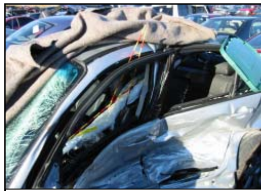
Figure 15. HPS air bag from outside.
