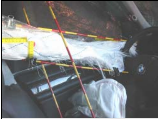
Figure 16. Damage from rescue personnel cutting the HPS air bag. Also, the air bag sustained minor cuts from contact with flying glass.
