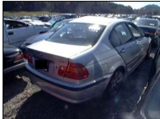
Figure 7. Rear area no residual damage from shrub impact.
