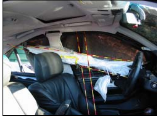
Figure 13. Deployed driver's HPS air bag.
