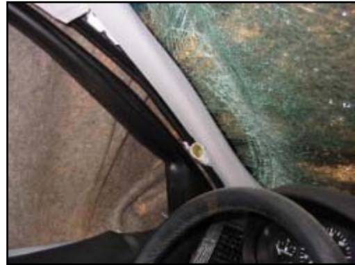
Figure 17. Area of HPS that rescue personnel cut.
