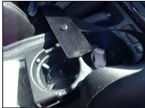
Figure 11. Cut lap belt portion remained buckled.
