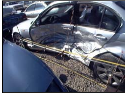
Figure 6. 2002 BMW 325i damage profile.
