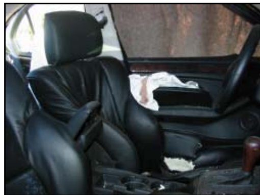
Figure 8. Intrusion into driver's position.
