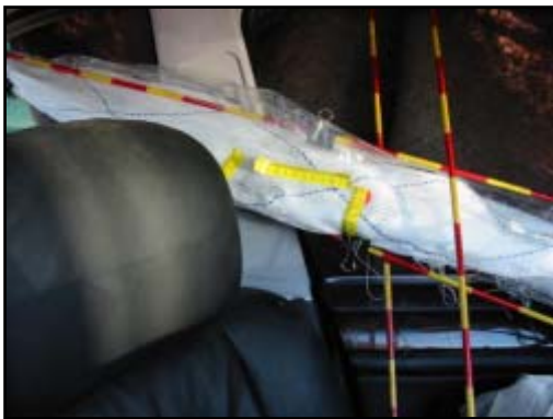
Figure 14. Head restraint contact to HPS air bag.
