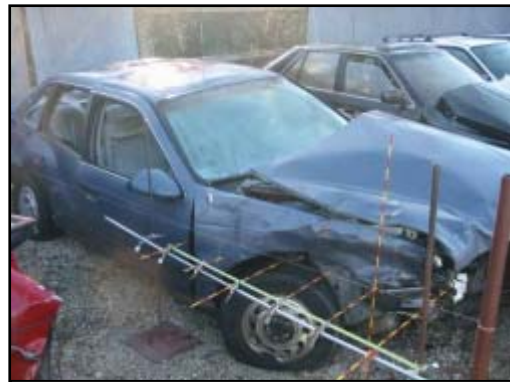
Figure 10. Right side damage from the initial impact with the Lexus.
