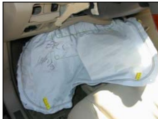
Figure 13. Deployed driver's knee bolster air bag.
