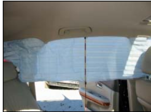
Figure 15. Deployed left side RSCA
