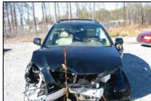
Figure 6. Frontal damage from the initial impact with the Ford.
