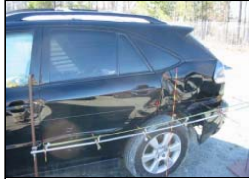
Figure 7. Left side damage from the secondary impact with the Ford.
