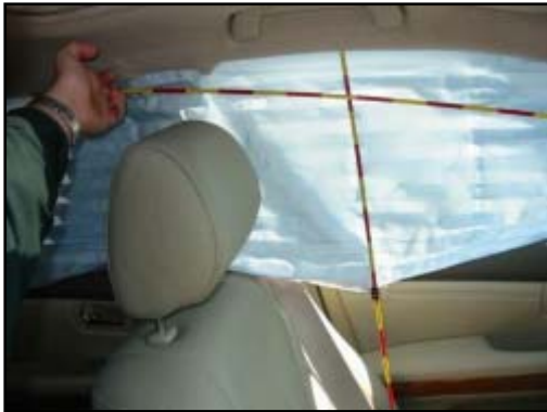
Figure 14. Deployed left side RSCA.
