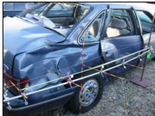
Figure 11. Right side damage from the secondary impact with the Lexus.
