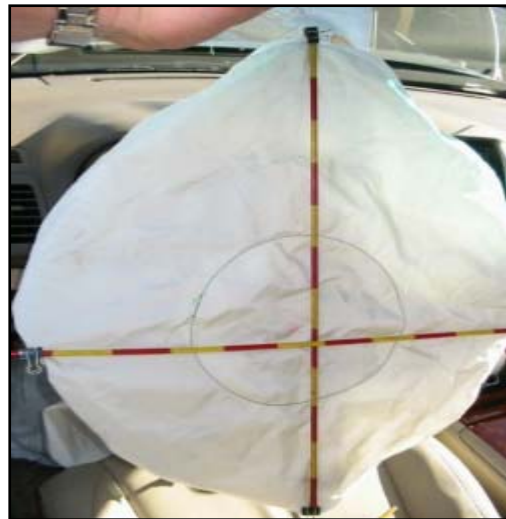
Figure 12. Deployed driver's frontal air bag.
