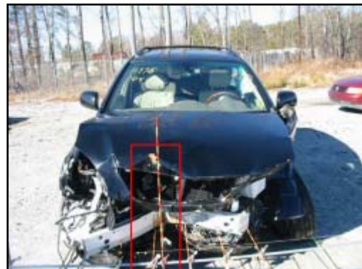
Figure 8. Damage from the impact with the tree.
