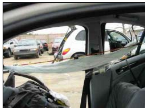
Figure 10. Deployed right side HPS air bag.
