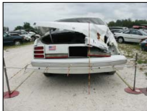
Figure 8. Damage area from impact with the Chevrolet.
