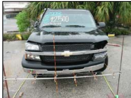
Figure 6. Damaged area from impact with the Oldsmobile.
