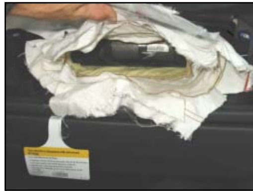
Figure 11. Front right air bag module. Note air bag was cut out prior to inspection.
