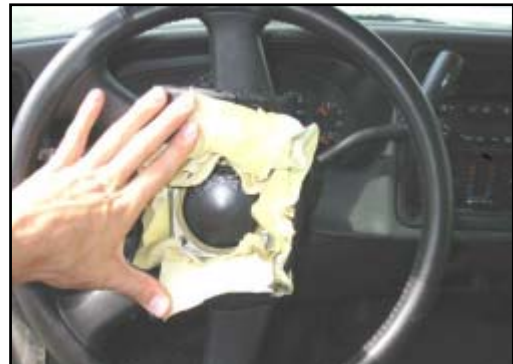
Figure 10. Driver's air bag module. Note air bag was cut out prior to inspection.
