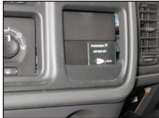
Figure 11. Front right air bag cut-off switch. Note the switch was keyed to the "Auto-On" position at the time of the NASS inspection.
