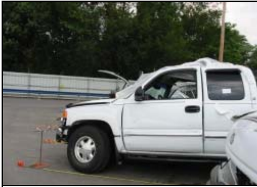
Figure 4. Sideswipe damage to front left half from hit and run vehicle. Note damage is under door panel trim.
