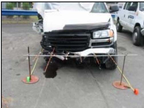
Figure 6. Frontal view of damage from pole impact.
