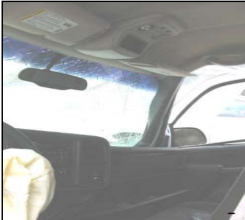
Figure 10. Non-deployed front right air bag.
