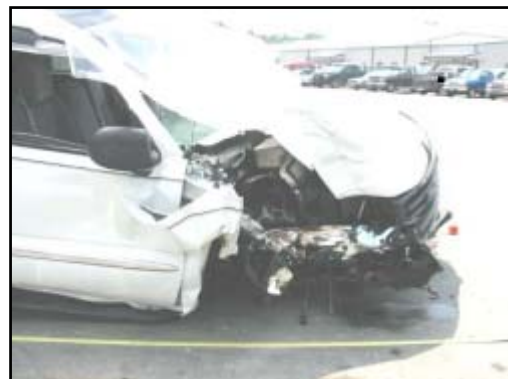
Figure 7. Damage to front right area from pole impact.
