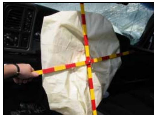
Figure 9. Deployed driver's frontal air bag.
