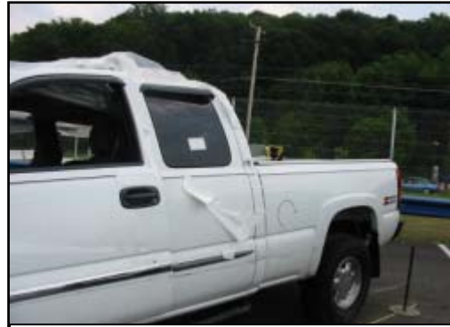
Figure 5. Sideswipe damage to rear left half from hit and run vehicle. Note damage is under door panel trim.
