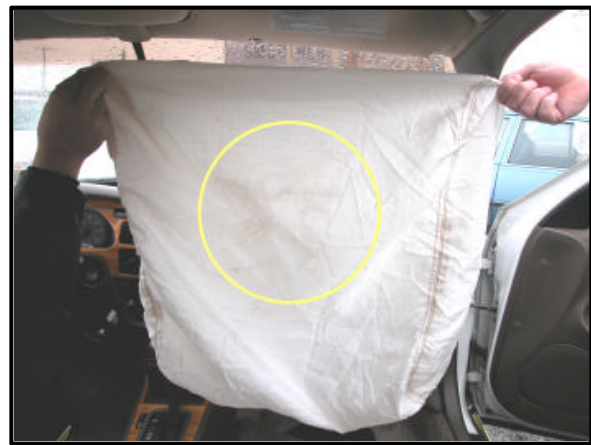
Figure 10: Contact evidence to the face of the air bag.
