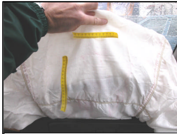
Figure 8: Contact to the bottom surface of the air bag.
